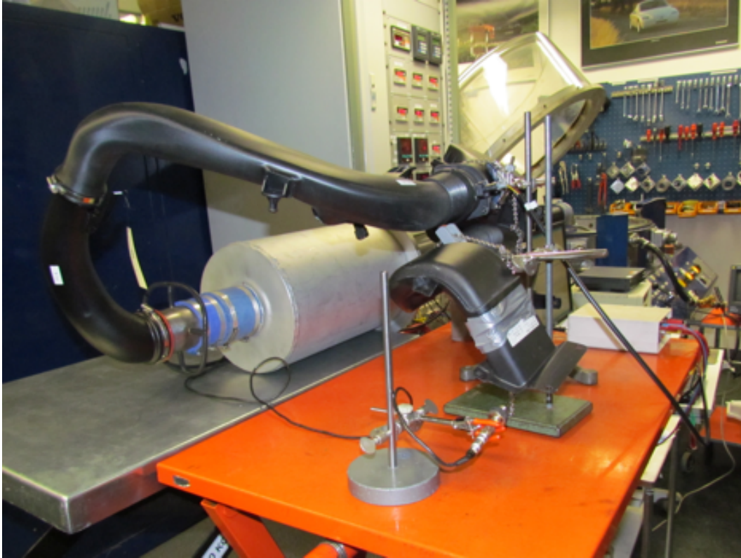
Figure 3.2.5: I5D P1 air induction system mounted in the flow rig
