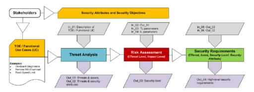
Figure 2.2: Workflow of HEAVENS security model
