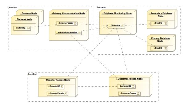
Figure 8: Home Sys deployment diagram  $\,$
