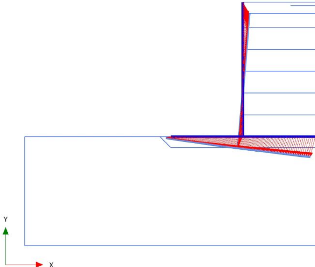
Figure 20 Wall displacements view tell direction and magnitude of displacement of the structure
