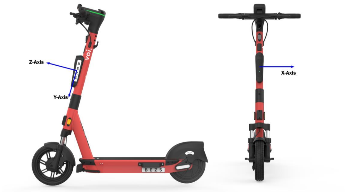
Figure 39 Co-ordinate system of the IMU and Gyroscope
