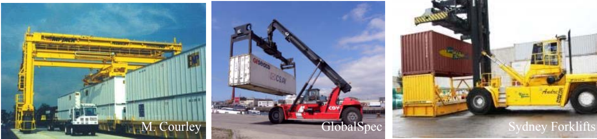
Figure 8: Transshipment equipment: gantry crane (left), reach stacker (middle) and a forklift (right).
