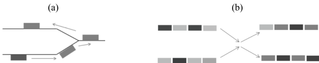
Figure 17: Depiction of shunting (a) and marshalling (b) operations
