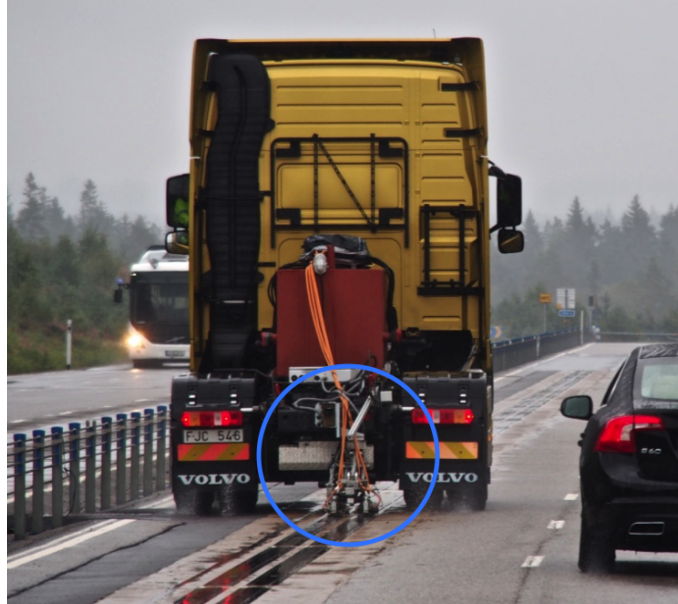
Figure 1.1. The robot arm shown in the circle, mounted on truck during testing. The two parallel tracks below the robot arm are the electrified tracks. Image from (Viktoria Swedish ICT 2014).
