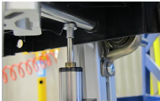
Figure A.4 Measurement of maximum displacement of beams at boundary.
