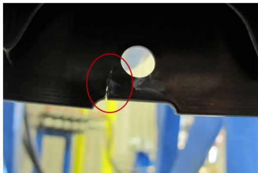
Figure 4.9 Deviating failure location at outer edge, failure at 727 594 cycles, load 210N.
