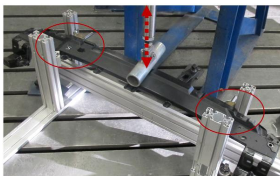
Figure 4.6 Three point bending test with force controlled cyclic loading and pinned boundary conditions.
