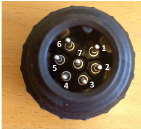
Figure 5.2: The figure illustrated the cable end from the TBR . The socket pins are defined in table 5.1 TBR [12].
