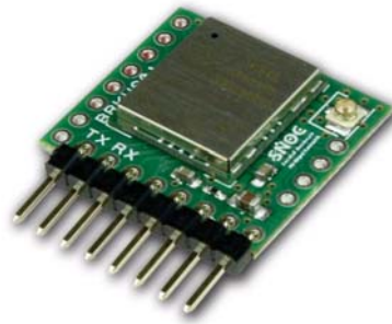
Figure 4.2: Illustration of a Sigfox breakout board BRKWS01 [16].
