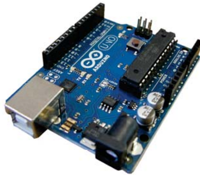
Figure 4.1: Illustration of an Arduino UNO board [24]
