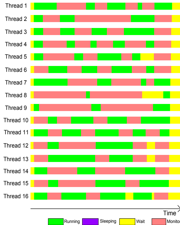
Figure 23: A snapshot displaying the 16 worker threads running with the old synchronization, a lot of waiting/holding locks (monitor) and a long execution time.
