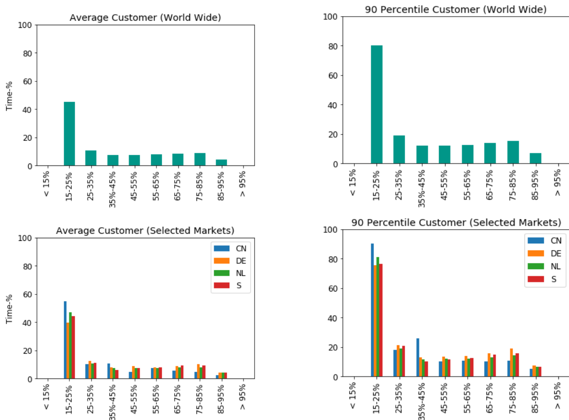
Figure 4.7: Time-% driven with different SoC-values for average and 90 th percentile customers - world wide and for China, Germany, Netherlands and Sweden.
