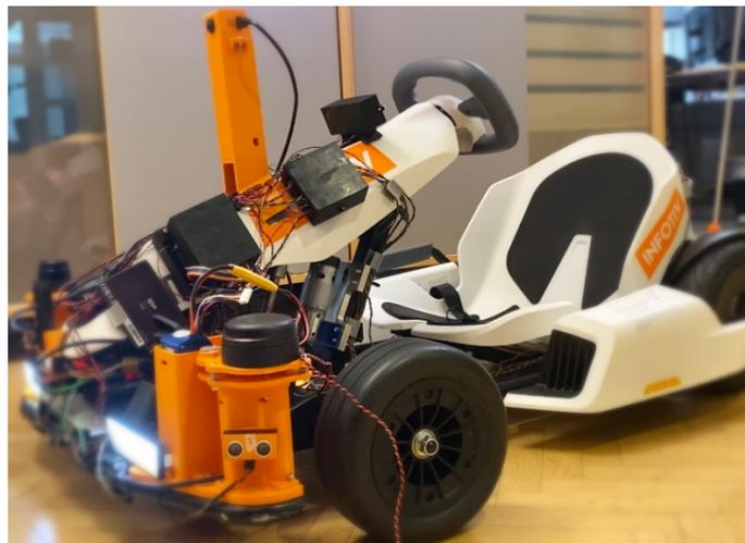
**Figure 3.1:** Image of Autonomous Platform third generation (AP3). It shows the current hardware, regarding sensors and computing units. Reprinted, with permission, from Infotiv AB
