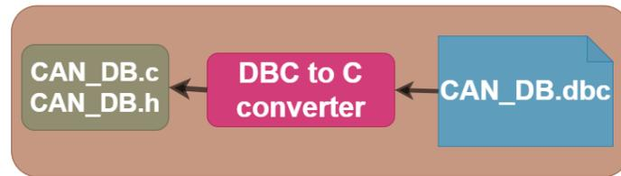
**Figure 6.4:** Conversion from CAN database to C code schematic flow is illustrated. The dbc file can be changed manually to add CAN frames and signals to the software. The DBC to C external library can be run by a developer when the dbc file has been changed to generate new C files with a specified structure containing every CAN frame and signal.
