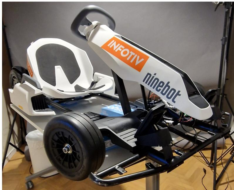
**Figure 3.2:** Ninebot S and Go-kart kit stock configuration Image of go-kart kit before AP4 implementation.
