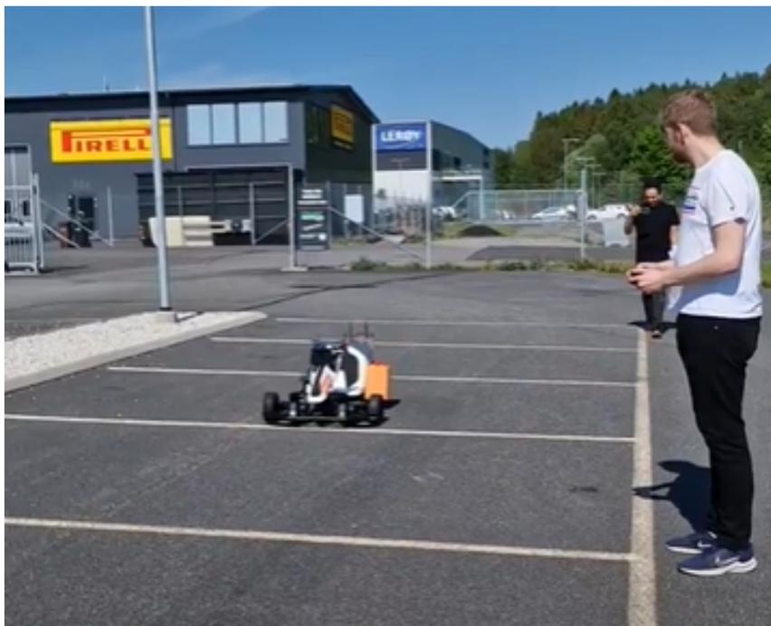
**Figure 7.7:** Driving AP4 on a parking lot, when measuring the brake distance of AP4, utilizing the known distance of each parking spot.
