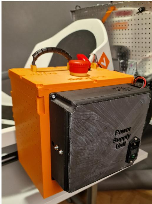
(a) Side view of power module with PSU mounted on the side.
