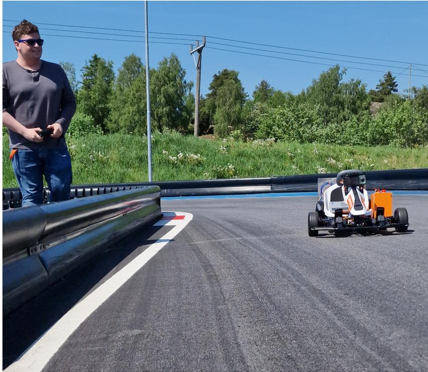
**Figure 7.6:** AP4 around the track, AP4 is controlled through a handheld Xbox controller, enabling drive-by-wire system. Complete a lap around the track on Gokart Centralen, Kungälv.
