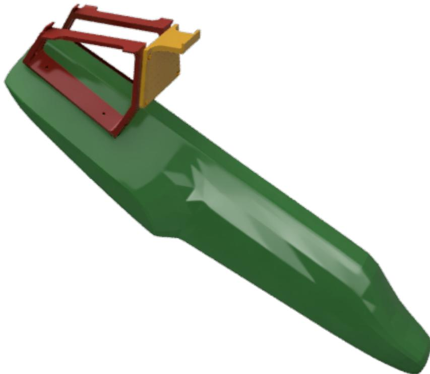
**Figure B.6:** Laptop holder, placed on the central panel of the go-kart.
