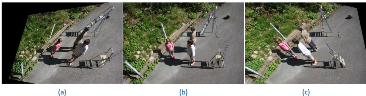
Figure 7. Homographic transformation of the views. (a), (b) and (c) are the left, center and right views respectively where (a) and (c) have been transformed to the ground plane of the middle view (b).
