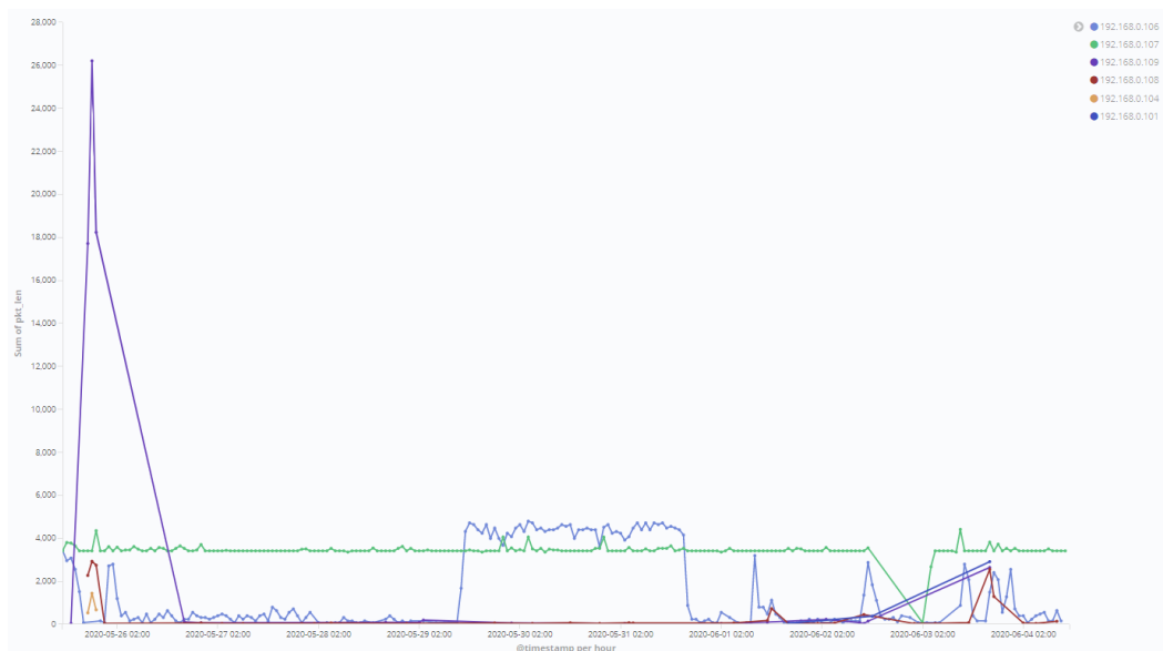
Figure 16: The sum of packet lengths (i.e. total bytes) per hour for all the devices in the well-known brands segment. The purple line corresponds to the Google Chromecast (192.168.0.109) and the green line the Google Home Mini (192.168.0.107).
