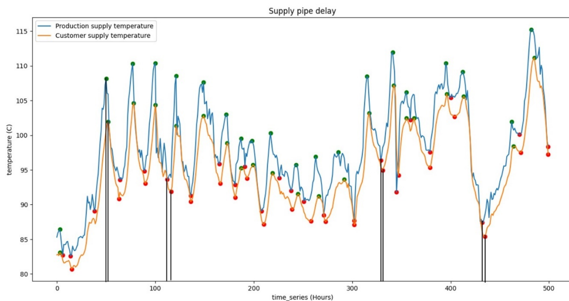
Figure 8 Peaks and valleys auto-detection by the model and delay calculation
