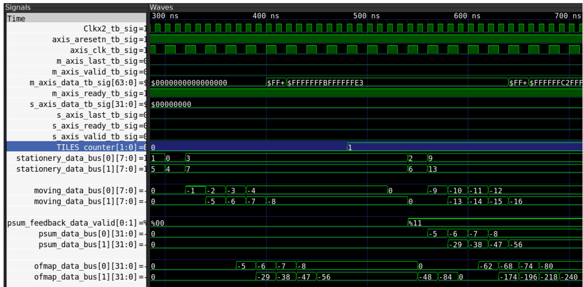
Figure 5.3: Top level simulation of M4K4N4 2x2 SA in Accelerator v2. Values are in hexadecimal on axis_data buses. Signals from the SA module is also seen on the figure which shows the first two tiles calculating the top rows of the result. Results for these signals are in signed decimal.
