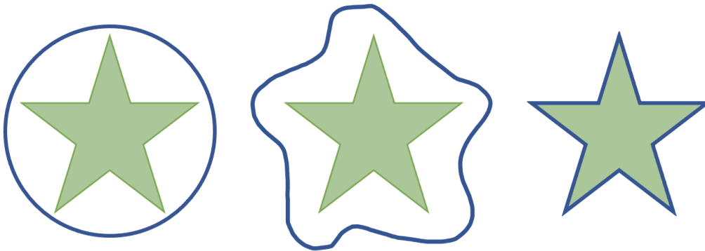
Figure 2.1: An illustration of the evolution of an active contour model fitting a snake to a star shape.
