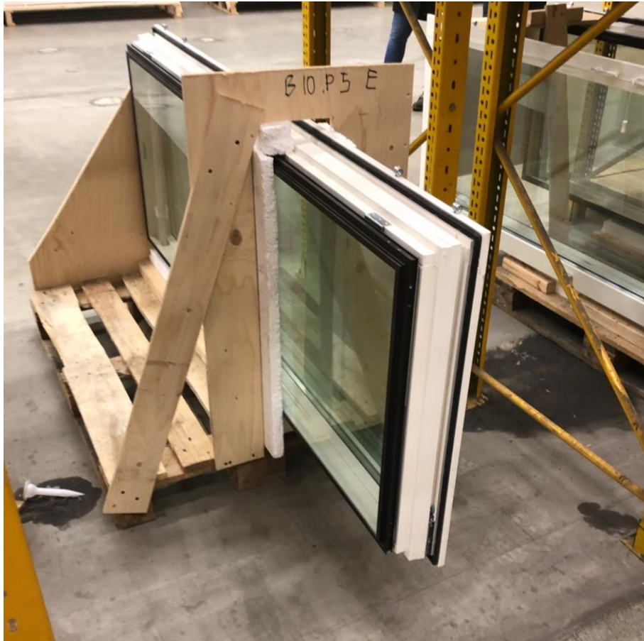
Figure 38: A delivery of a window with only half the window secured on a pallet, which increases the risk for transportation damages.
