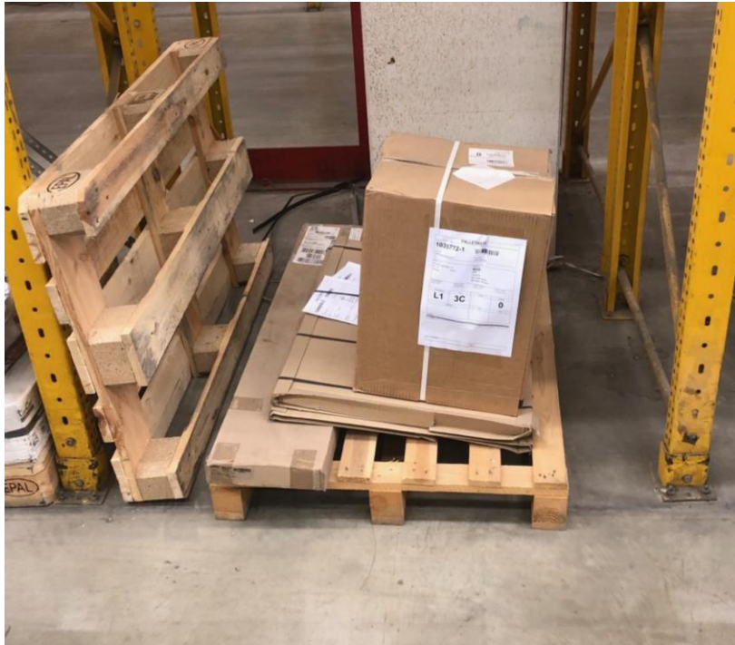
Figure 35: Storage of material without securing the goods, the packages can easily fall off the pallet and cause transportation damages.
