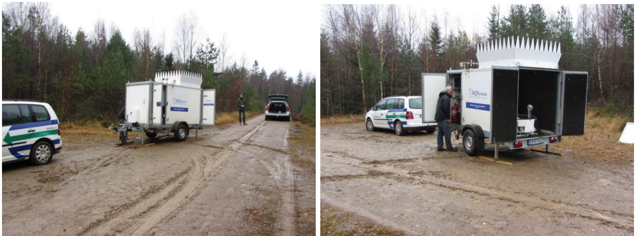
Figure 6.2: Installation of the BRN SODAR.
