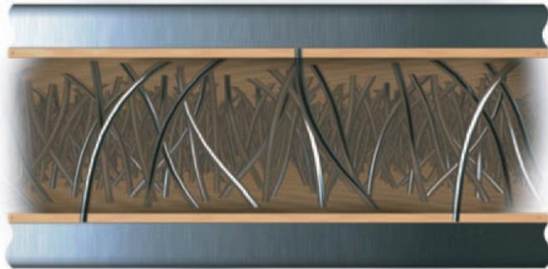
Figure 1.3 a). A cut-through of Hybrix where the different layers are visible.
