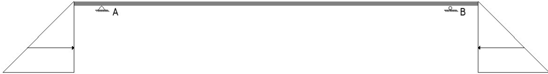
Figure 3.14: Earth pressure at rest acting on the end shields.
