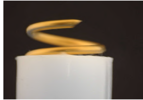
(d) An image of a moving electrode captured by a camera with rolling shutter.
