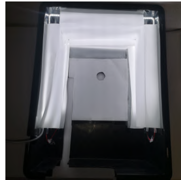
(f) The final lighting box with diffusion filter covering the light.
