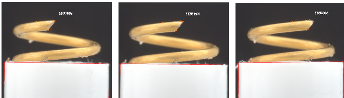
(a) The spiral tip is rotated too far to the left. (b) The spiral tip is rotated correctly. (c) The spiral tip is rotated too far to the right.
