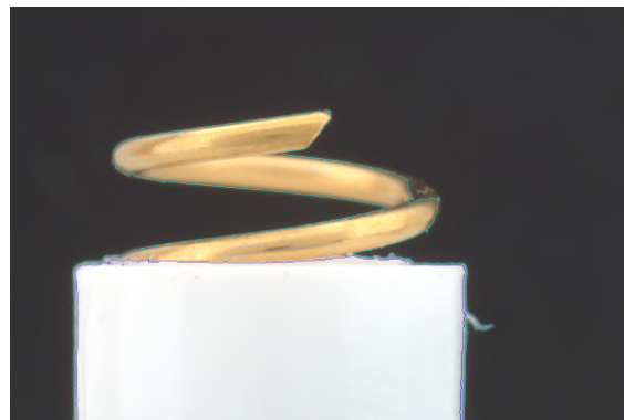
(d) The placement of electrode 25, when measuring an angle of 45.3^\circ
