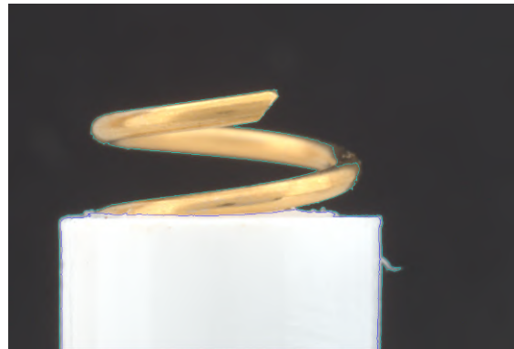
(b) The placement of electrode 25, when measuring an angle of 41.8^\circ
