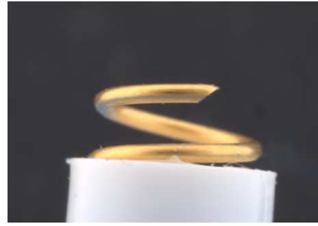
(b) An image of a moving electrode captured by a camera with global shutter.
