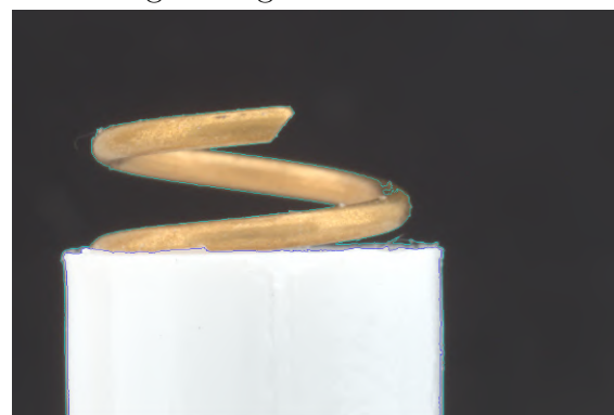
(d) The placement of electrode 24, when measuring an angle of 46.2^\circ
