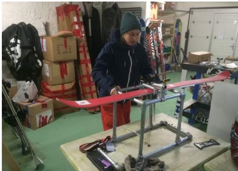
Figure 29. Testing the flex of the skis with a flex rig that was built for this project
