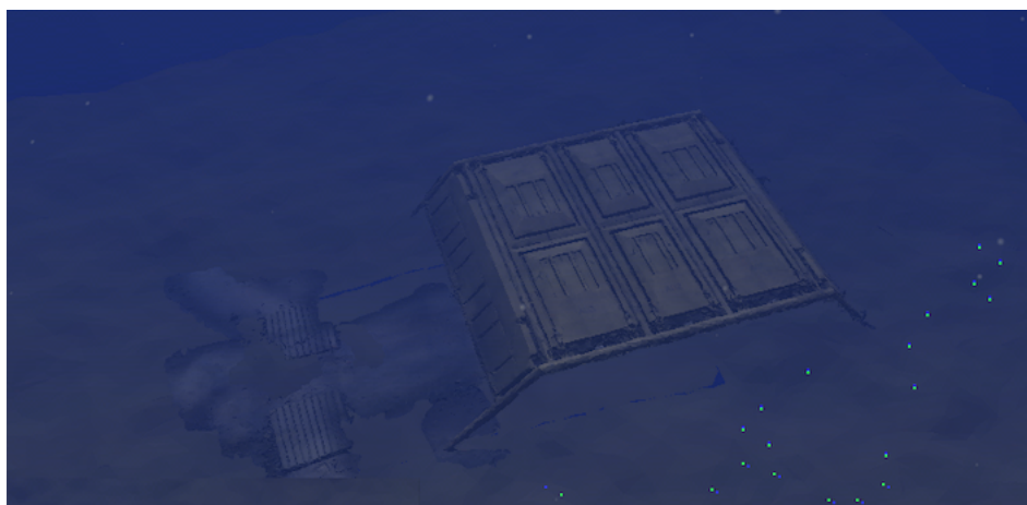
Figure 5.1: Subseafloor and template taken from the real world 3D cloud point and imported into an underwater simulator.
