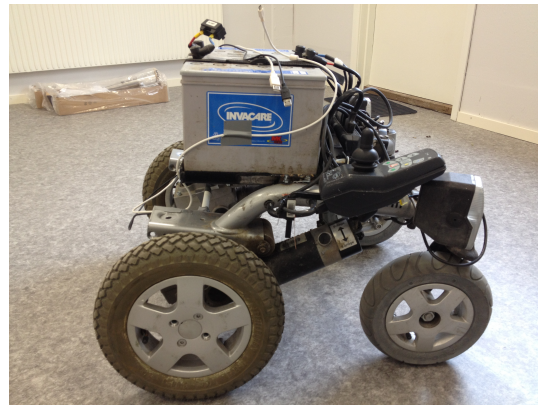
Figure 2.5: The stripped and modified power-driven wheelchair.
