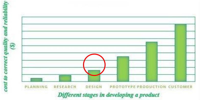
Figure 25: Impact of opportunity of defects in different stages of developing a product.
