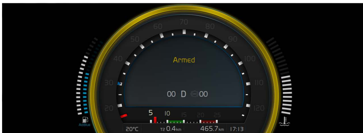
Figure 36: The instrument cluster visualisation of the Armed State with automated switch activated
