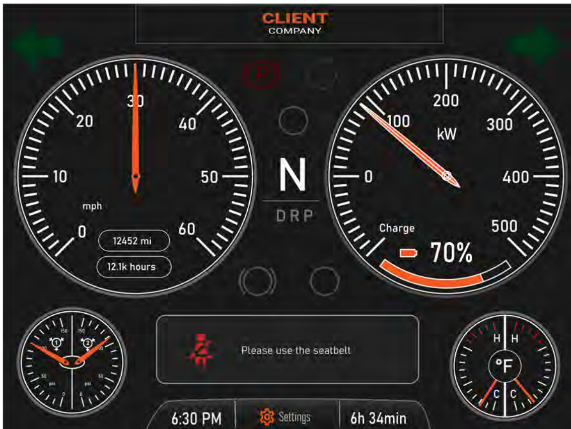
Figure 10.2: Concept 1 from Iteration I. This concept focused on preserving analogue gauges from the traditional terminal tractor dashboard interface. [Authors contribution]
