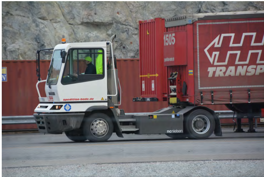
Figure 2.1: Terberg terminal tractor, Stockholm Nord Container Terminal, Sweden. [Beng Oberger, CC BY-SA 4.0, via Wikipedia Commons]
