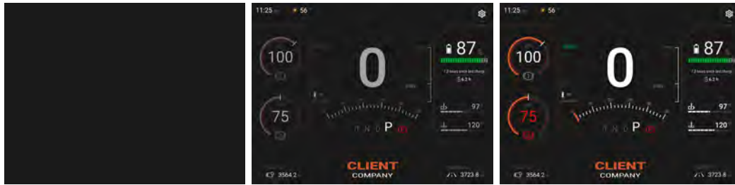
Figure 7.20: The three stages of ignition that we proposed during the second iteration of the process. In the leftmost image, the display is completely dark, symbolising that the tractor is turned off. The centre image displays a greyed-out interface, which symbolises that the low-voltage system is active. The rightmost image displays the interface once the high-voltage system is active, which returns the colour to the interface. [Authors contribution]
