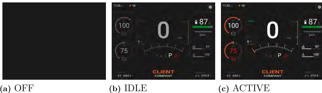
Figure 9.10: The three stages of the interface, namely OFF, IDLE, and ACTIVE. The interface is OFF when the tractor is off, in IDLE when its turned on but the high-voltage inactive, and ACTIVE once the high-voltage is active. [Authors contribution]
