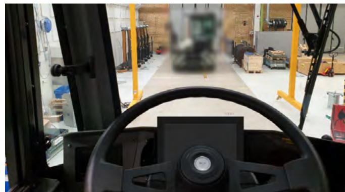
Figure 7.12: Estimation of how our proposed screen placement will look like from the user's point of view, the steering wheel is in uppermost position. Although parts of the display remain obstructed, drivers would be able to lean to view the rest of the interface. Furthermore, we could refrain from placing important information and gauges in these obstructed sections. [Authors contribution]
