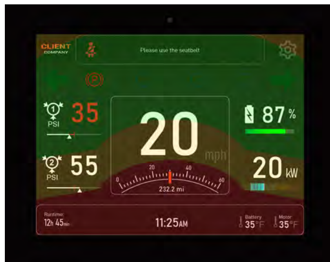
Figure 7.14: Heat map of the worst-case visibility if the interface would be raised and integrated with the dashboard. The red areas are sections of the interface that some users may never see, even if they move slightly, yellow indicates sections of the screen that would be somewhat obstructed, but observable, and green indicates sections with good visibility for the vast majority of users. [Authors contribution]
