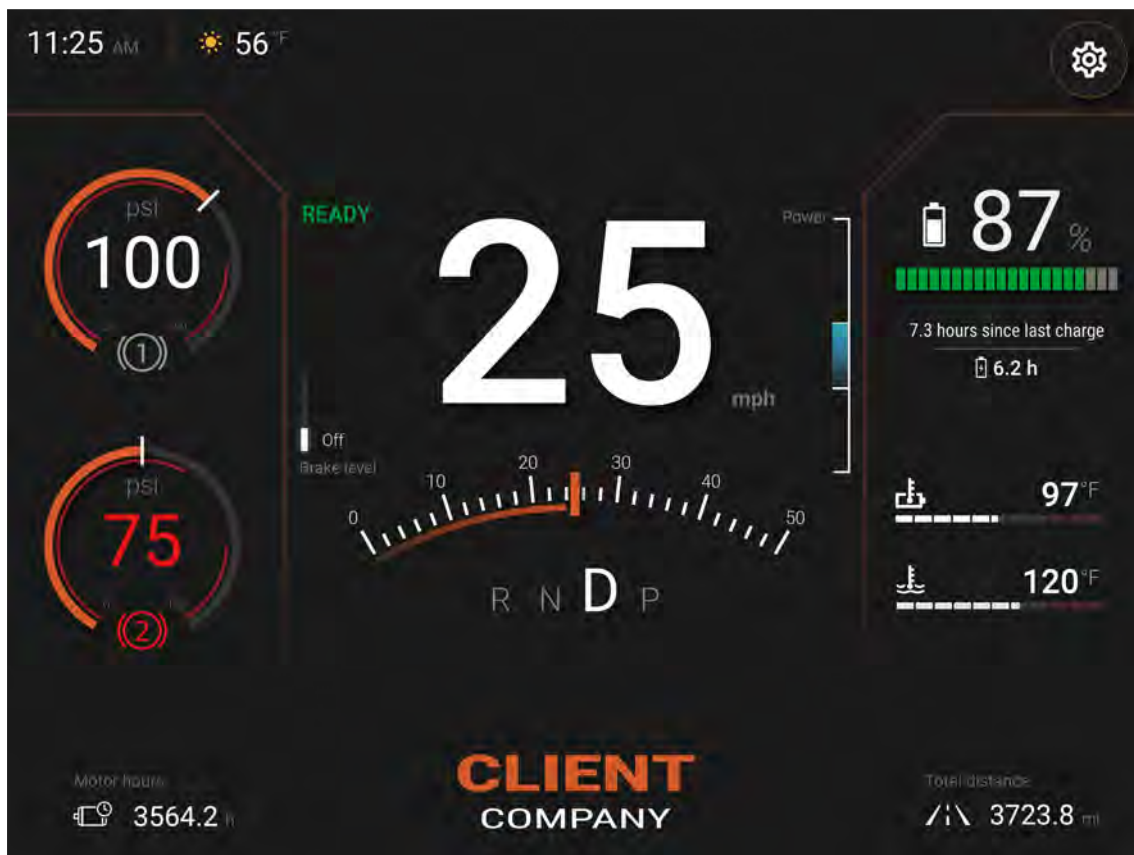
Figure 9.1: The final concept for an electric terminal tractor dashboard display. This is the same design as in Iteration III, and how it was evaluated in Chapter 7 - Evaluate . [Authors contribution]
