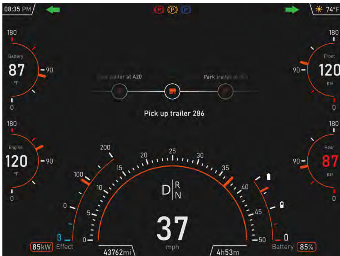
Figure 10.5: Concept 4 from Iteration I. This concept speculates how a fleet management system could be incorporated in a terminal tractor dashboard interface, taking up a central location in the interface. [Authors contribution]
