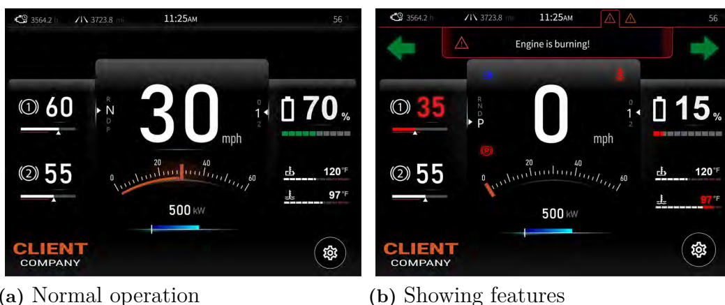
Figure 7.22: Concept 1 out of the three concepts created in Iteration II. The left image depicts how it will appear in a normal operating state, the right image is created to show additional features such as tell-tales and critical values. [Authors contribution]
