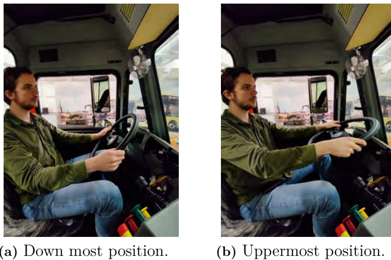
Figure 7.9: Two images that show the different steering wheel configurations available to drivers in the new terminal tractor. The uppermost configuration in (b) is more spacious than the down most configuration in (a), although it further obstructs the view of the dashboard display, as can be seen in Figure 7.10. [Authors contribution]
