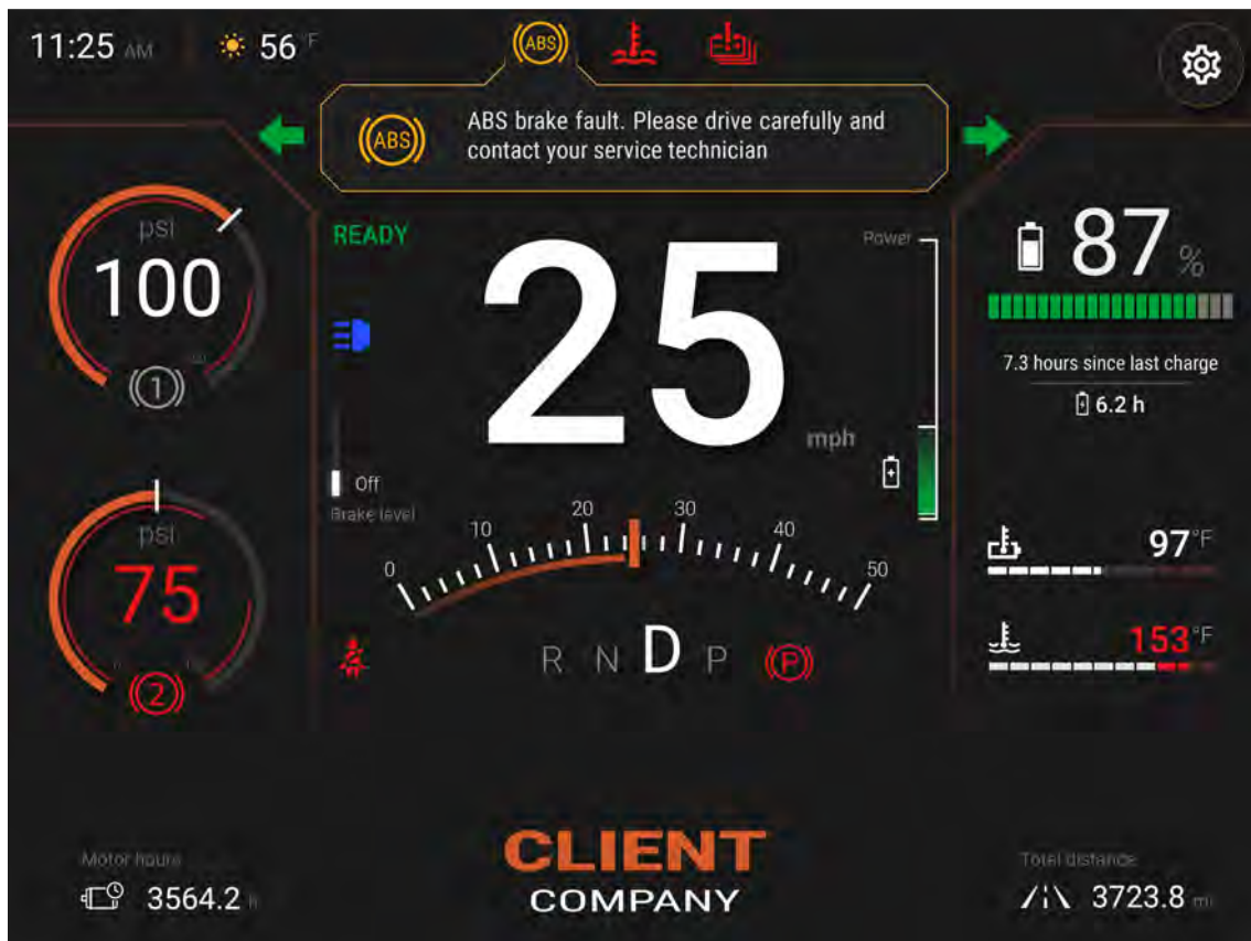
Figure 9.2: The final concept. In this Figure additional elements that are hidden during normal operation are presented. [Authors contribution]
