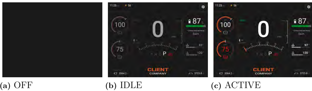
Figure 7.25: Three images that show the three different states for the interface; OFF is when the terminal tractor is turned off, IDLE is for when the low-voltage is turned on, and ACTIVE is when the high-voltage that drives the motor is on. [Authors contribution]
