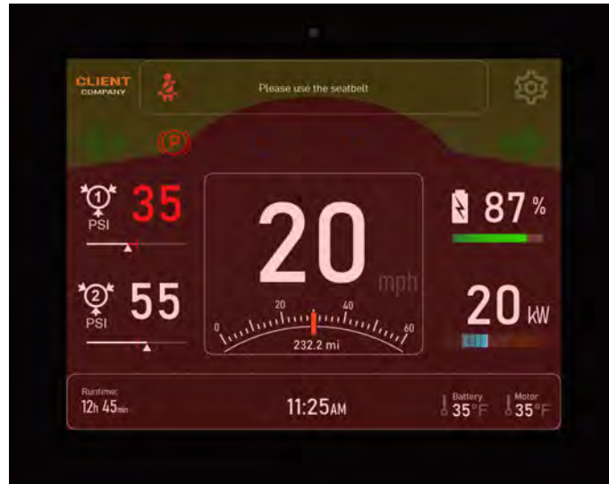
Figure 7.13: Heat map of the worst-case visibility if the interface would remain in the location at the time of our study. The red area is the section which some drivers may never see, even if they make small movements. [Authors contribution]
