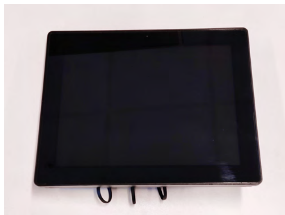
Figure 2.3: The screen that will be used in the final product for the interface, which is 11". The placement in the dashboard is not decided by the project stakeholder but is assumed to be somewhere behind the steering wheel. [Authors contribution]
