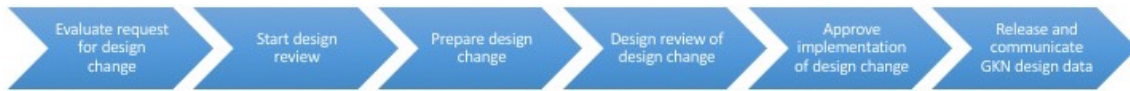
Figure 4.2: The EC process at GKN. Authors' own figure, based on the OMS at GKN.
