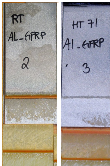
Figure 4.4: Comparison between a cohesive and adhesive fracture surface after tensile shear testing between GFRP to aluminium. Left part of figure is test sample 2 at RT testing and shows cohesive failure. Right part of figure is test sample 3 at elevated temperature, shows adhesive failure.
