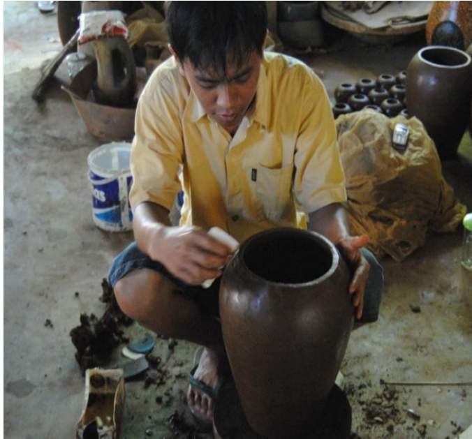
Figure 3: Preparation of green body.
