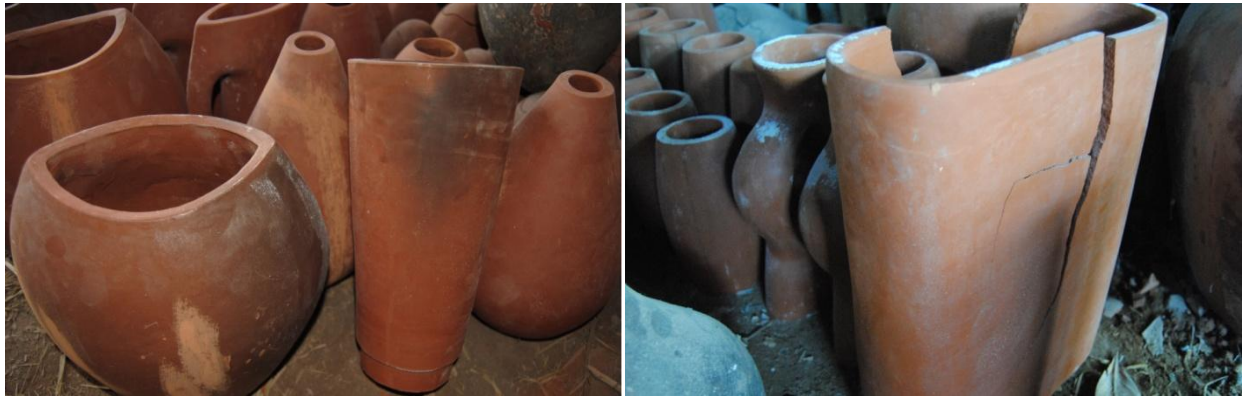
Figure 20: The clay bodies after burning process.
