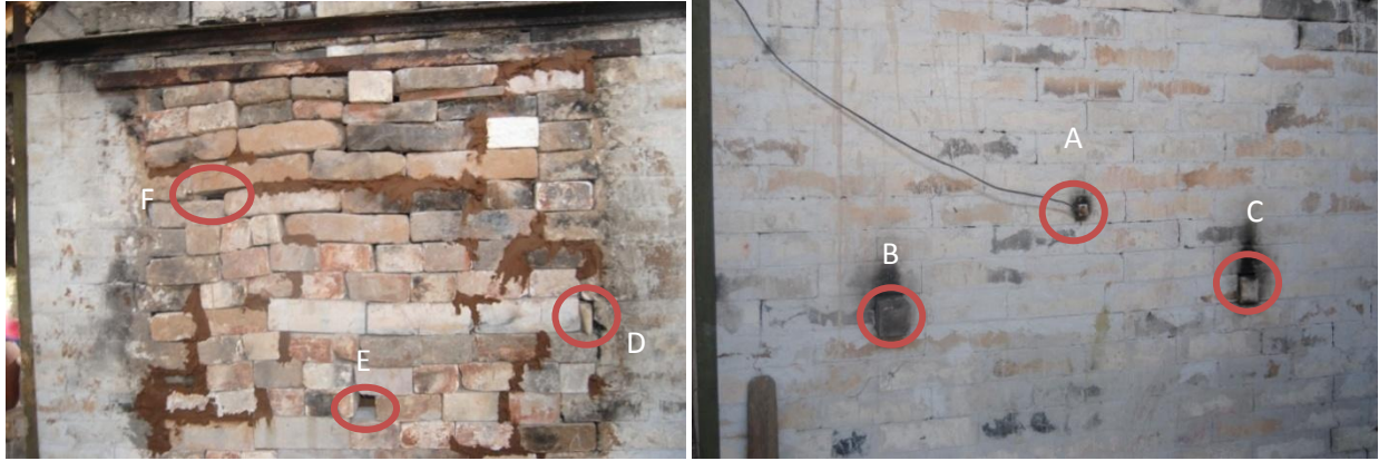
Figure 8: Temperature measurement points. To the left, the points in front of the kiln and to the right, the points in the back side are shown.
