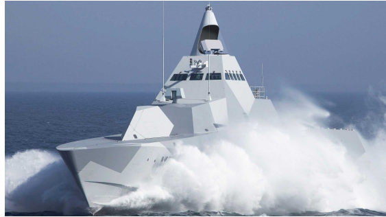
(b) The Sea Giraffe AMB with the radar antenna located inside the cone on top of the vessel.
