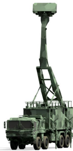
(a) The Giraffe AMB with the radar antenna located at the top.
