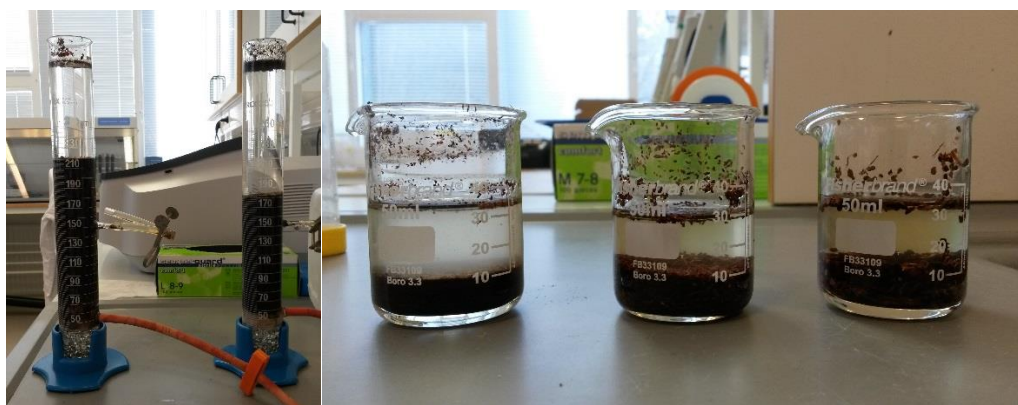
Figure 6 Left: Glass columns used for laboratory testing of the hydraulic rate. Right: Peat and bark completely saturated in water.
