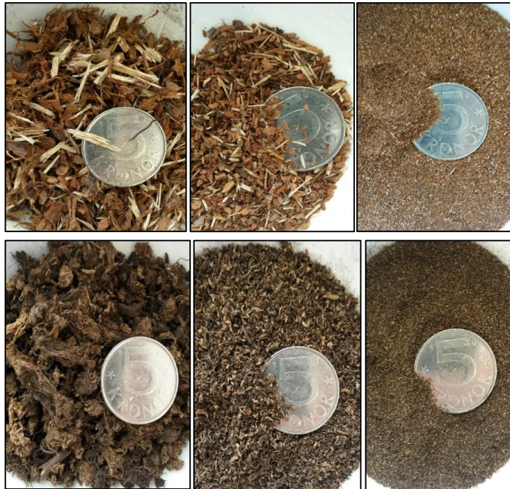
Figure 7. The >2 mm, 0.5 - 2 mm and <0.5 mm fractions of the peat and the bark.
