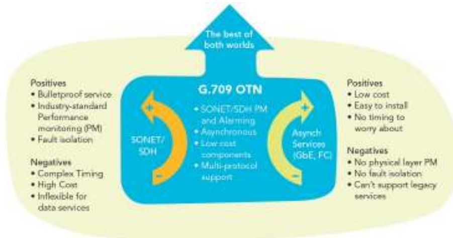
Figure 2-7: Advantages of OTN format [The Value of OTN for Network Convergence and IP/Ethernet Migration]
