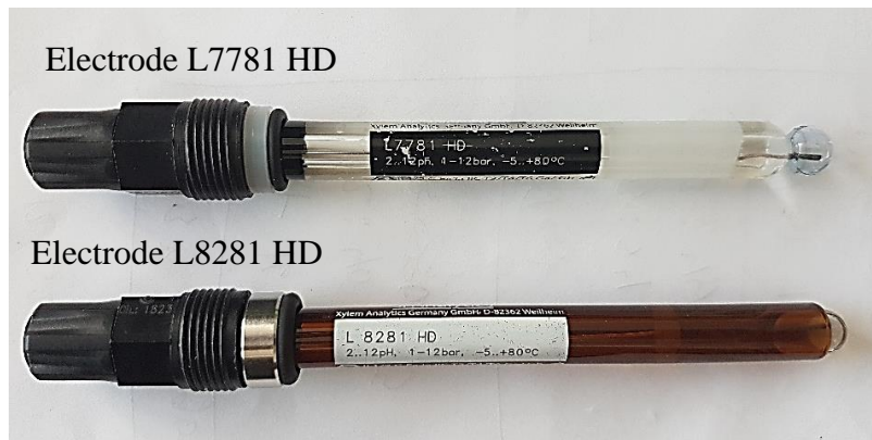
Figure 9: Sensors used in the experiment for measuring pH, product of Xylem Inc.
