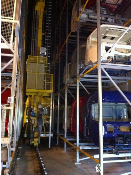
Figure 3. S/RM transporting a cab.
