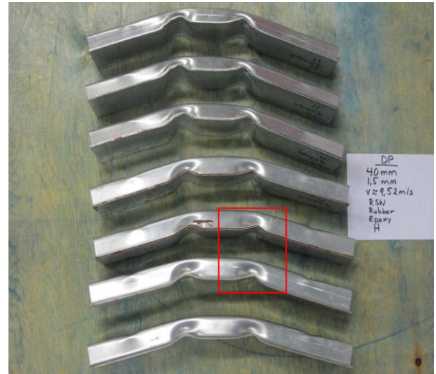
Figure 4.20: DP600, 1,5 mm thick, 40 mm spot weld spacing, high deformation. From top: 3 RSW, 2 rubber and 2 epoxy weld bonded.
