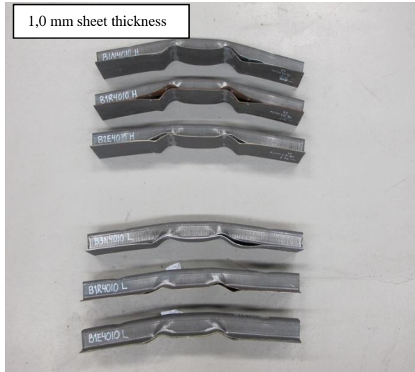
Figure 4.38: Usibor beams with thickness 1,0 mm. From top: RSW, rubber weld bonded and epoxy weld bonded, both high (upper group) and deformation (lower group)
