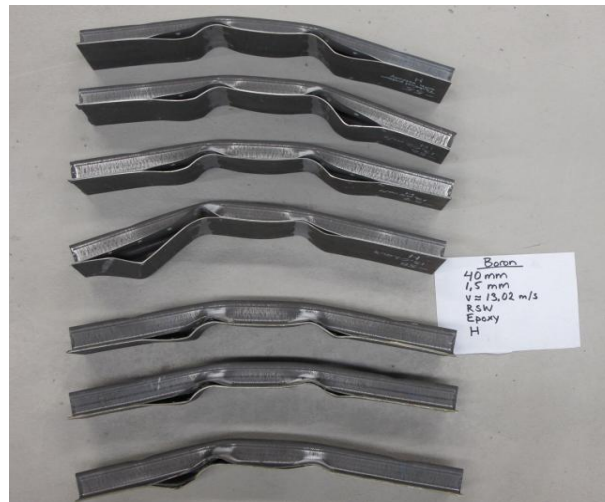
Figure 4.33: Usibor, 1,5 mm thick, 40 mm spot weld spacing, high deformation. From top: 3 RSW, 3 rubber and 3 epoxy weld bonded.
