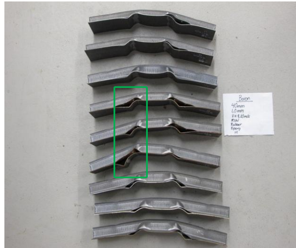
Figure 4.31: Usibor, 1,0 mm thick, 40 mm spot weld spacing, high deformation. From top: 3 RSW, 3 rubber weld bonded and 3 epoxy weld bonded.
