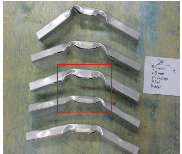
Figure 4.16: DP600, 1,0 mm, 80mm spot weld spacing, high deformation. From top: 3 RSW and 2 rubber weld bonded
