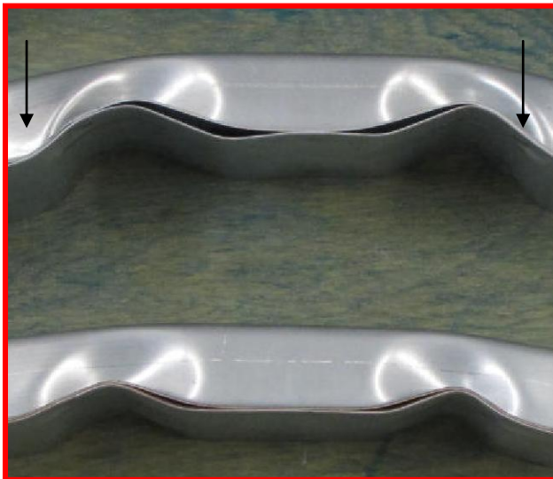
Figure 4.17: Magnified picture of the separation at low deformation. From top: RSW and rubber weld bonded.
