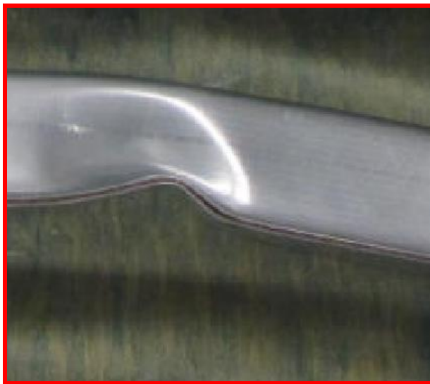
Figure 4.13 The rubber adhesive starts to separate at the hit points of the impactor.
