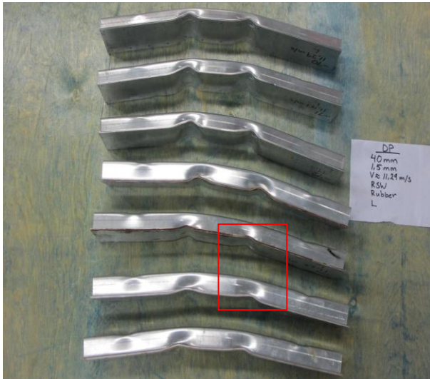
Figure 4.19: DP600, 1,5 mm thick, 40 mm spot weld spacing, low deformation. From top: 3 RSW, 2 rubber and 2 epoxy weld bonded.
