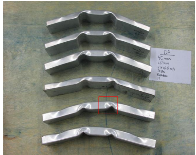
Figure 4.12. DP600, 1,0 mm, 40 mm spot weld spacing, high deformation. From top: 3 RSW and 3 rubber weld bonded
