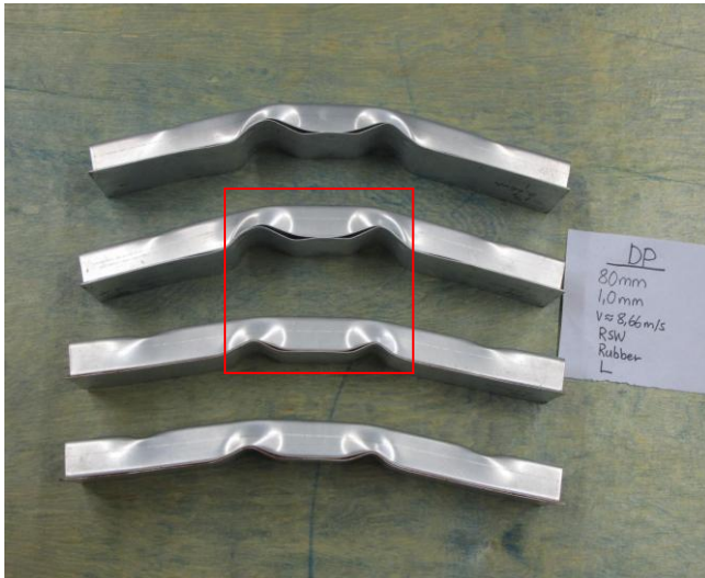
Figure 4.15: DP600, 1,0 mm, 80mm spot weld spacing, low deformation. From top: 2 RSW and 2 rubber weld bonded
