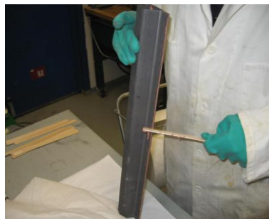
Figure 3.8: Wiping off the excess adhesive
