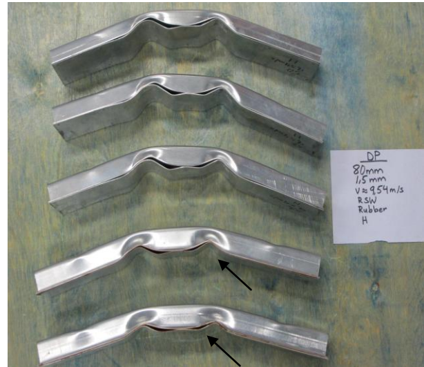
Figure 4.24 : DP600, 1,5 mm thick, 80 mm spot weld spacing, high deformation. From top: 3 RSW and 2 rubber weld bonded.
