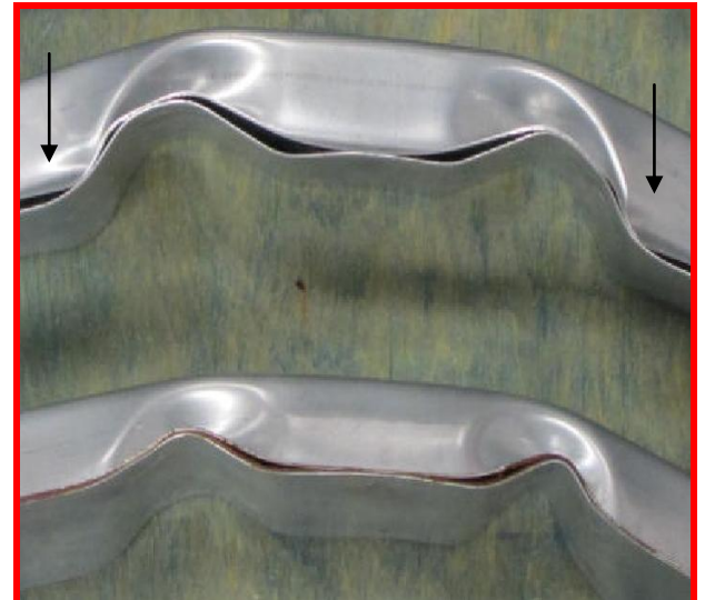
Figure 4.18: The RSW-beams separate more than rubber weld bonded beams at high deformation. From top: RSW and rubber weld bonded.
