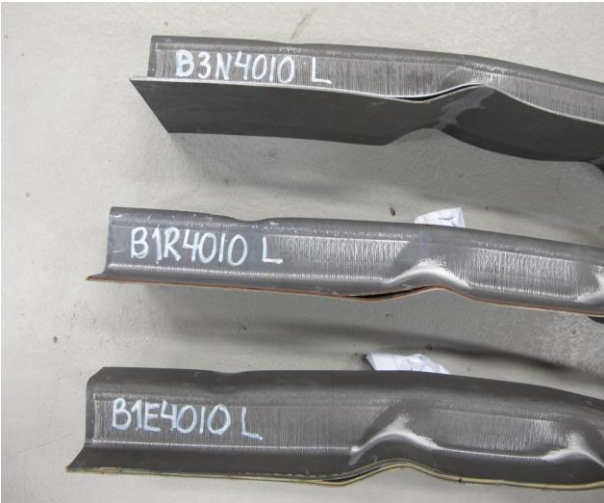
Figure 4.34: Usibor, 1,0 mm thick, 40 mm spot weld spacing, low deformation. From the top: RSW, rubber weld bonded and epoxy weld bonded.
