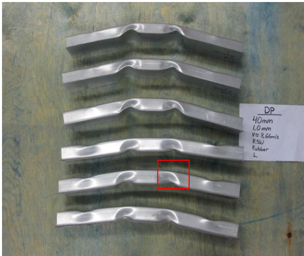
Figure 4.11. DP600, 1,0 mm, 40 mm spot weld spacing, low deformation. From top: 3 RSW and 3 rubber weld bonded
