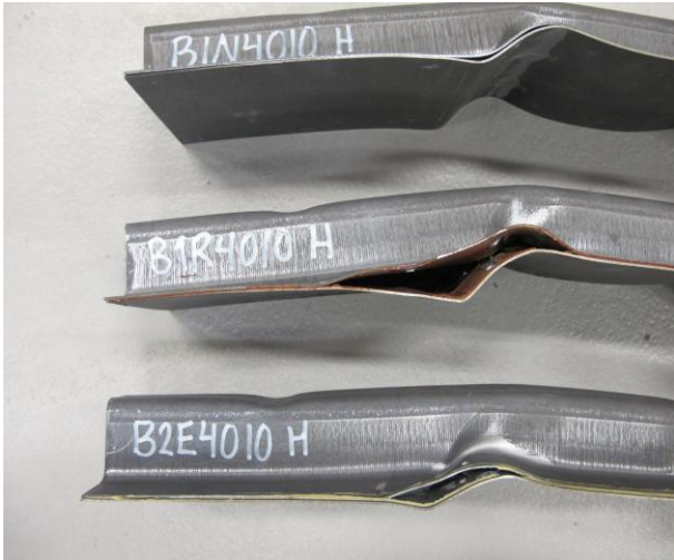
Figure 4.35: Usibor, 1,0 mm thick, 40 mm spot weld spacing, high deformation. From the top: RSW, rubber weld bonded and epoxy weld bonded.
