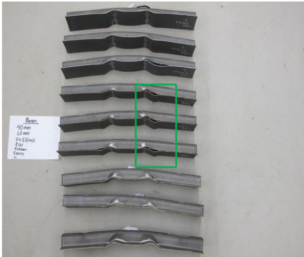
Figure 4.30: Usibor, 1,0 mm thick, 40 mm spot weld spacing, low deformation. From top: 3 RSW, 3 rubber weld bonded and 3 epoxy weld bonded.
