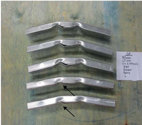
Figure 4.23: DP600, 1,5 mm thick, 80 mm spot weld spacing, low deformation. From top: 3 RSW and 2 rubber weld bonded.
