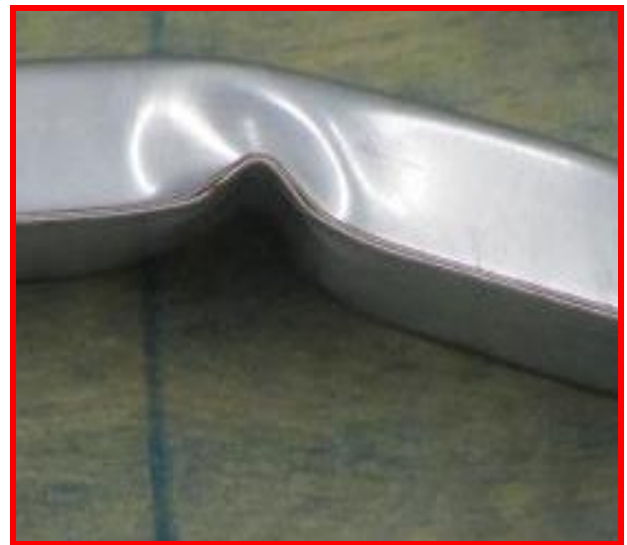
Figure 4.14 The rubber adhesive is still stable and no separation in the flanges was observed.
