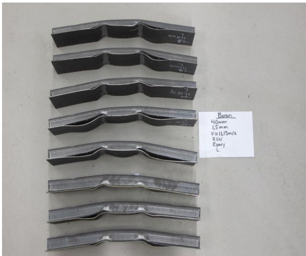
Figure 4.32: Usibor, 1,5 mm thick, 40 mm spot weld spacing, low deformation. From top: 5 RSW and 3 epoxy weld bonded.
