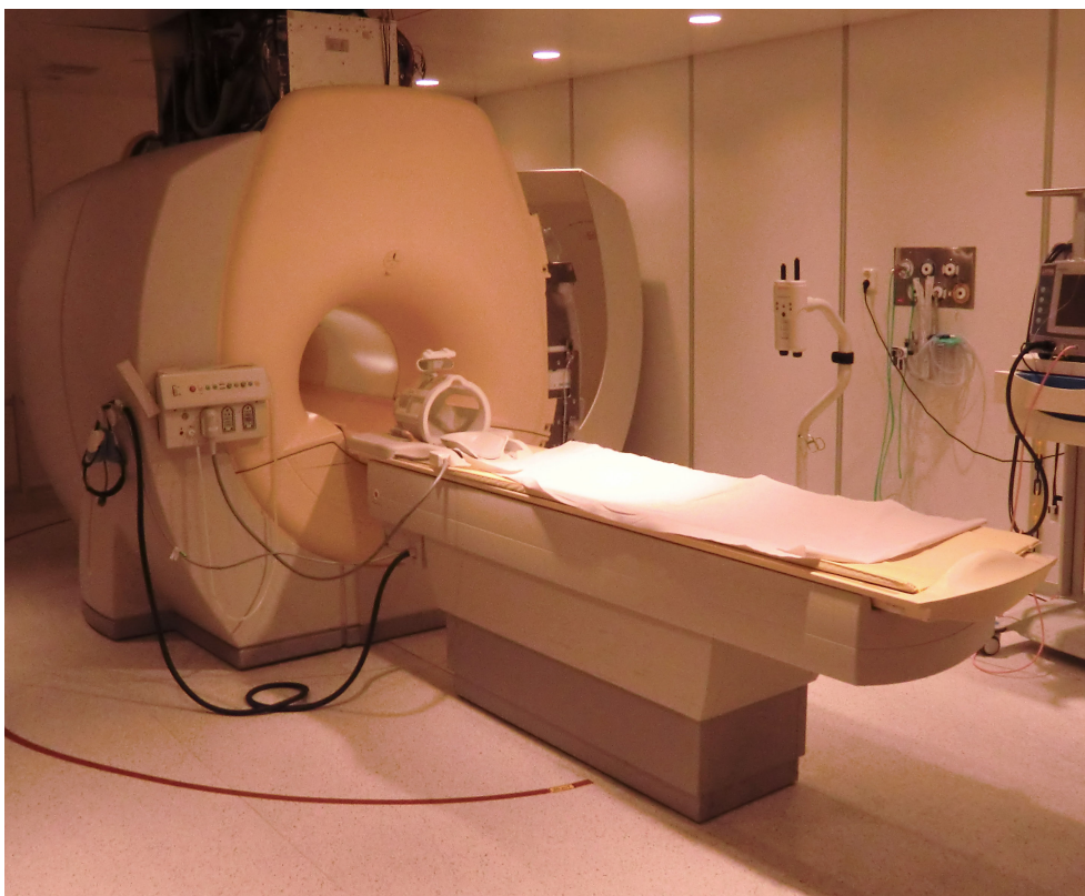
Figure 1.1: The 3T Philips MRI scanner that was used to generate all the images used in this thesis. The scanner is fitted with the receiving head coil that was used for imaging of both the phantom and the volunteers.
