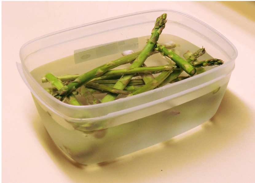
Figure 4.6: The phantom used to generate real image data to test the correction method. It consists of asparagus stems placed in water, which gives it both a distinct structural contrast and a directionally varying diffusion sensitivity. This makes it a perfect phantom for testing eddy current distortion. A plastic lid was placed on the container before it was put in the MRI scanner.
