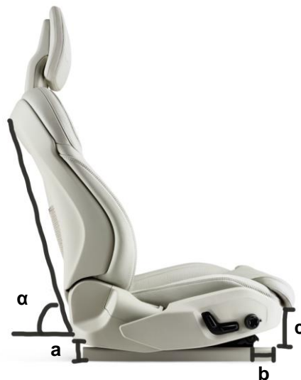
Figure 3.6. Seat design position used in experiment B-F. \alpha is the backrest angle, a and c is the height adjustments in the back and front, and b is the length adjustment in the front.
