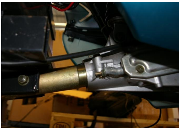
Figure 28 The joint system of Xingyue DM82.
