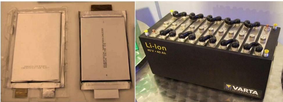
Figure 15 Li-ion battery, left: cell, right: battery pack.
