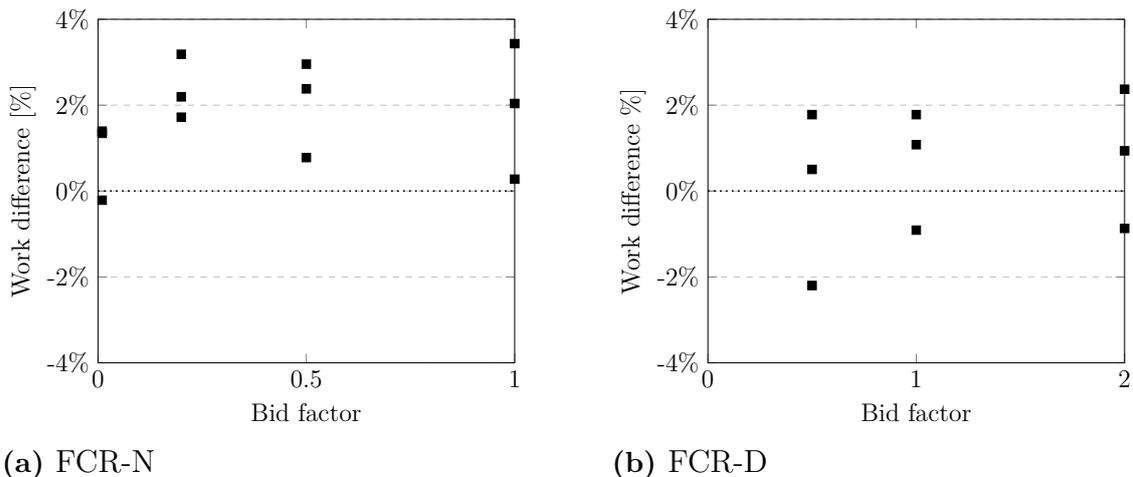
**Figure 4.3:** Difference in performed work compared to without FCR activation (average per day and forklift) for different bid factors. (Note that each case were simulated 3 times with different results due to the randomness of the model.)
