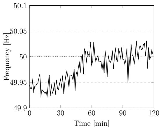
**Figure 2.3:** Example of frequency fluctuations during two hours in January 2017. (Data from 170101 00:01-02:00, provided by Svenska Kraftnät on request.)
