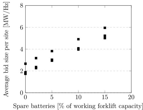
**Figure 4.4:** Average bid size per day and site for FCR-N and different spare battery capacities. Note that the capacity bid in [MW/Hz] is 10 times as high as the available capacity. (Also note that each case was simulated 3 times with different results due to the randomness of the model.)
