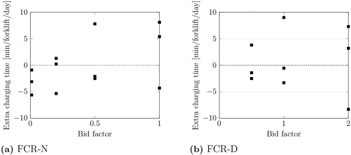
**Figure 4.1:** Extra charging minutes for different bid factors in the base case. (Note that each case was simulated 3 times with different results due to the randomness of the model.)
