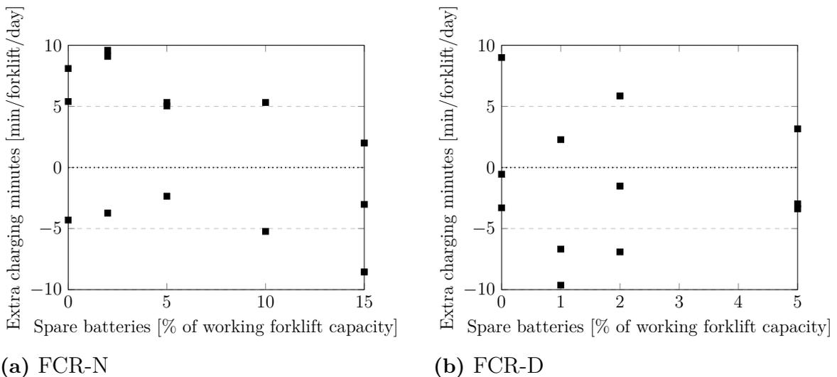
**Figure 4.5:** Extra charging minutes for different spare battery capacities. (Note that each case was simulated 3 times with different results due to the randomness of the model.)
