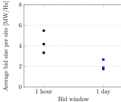
**Figure 4.7:** Average bid size (average per day and site) calculated from forklift site model for FCR-N with bid windows of 1 respectively 24 hours. (Note that each case was simulated 3 times with different results due to the randomness of the model.)
