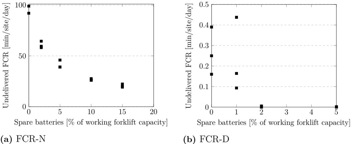
**Figure 4.6:** Number of minutes per day in which requested FCR power failed to be delivered for different spare battery capacities. Note the scale difference between the two plots. (Also note that each case was simulated 3 times with different results due to the randomness of the model.)
