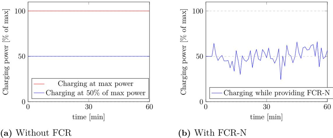
**Figure 2.6:** Illustrative example of how charging power might look like without respectively with FCR-N activation (Calculated using 50% of maximum charging power as FCR-N capacity bid, using frequency data provided by Svenska kraftnät.)
