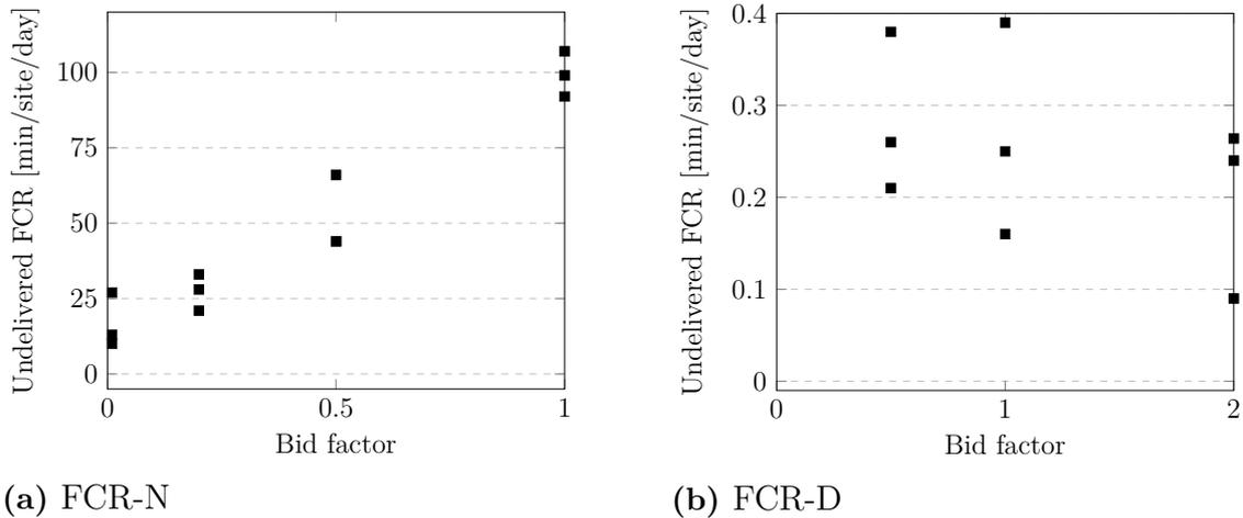
**Figure 4.2:** Number of minutes per day and site in which requested FCR power failed to be delivered for different bid factors. Note the scale difference between the two plots. (Also note that each case was simulated 3 times with different results due to the randomness of the model.)
