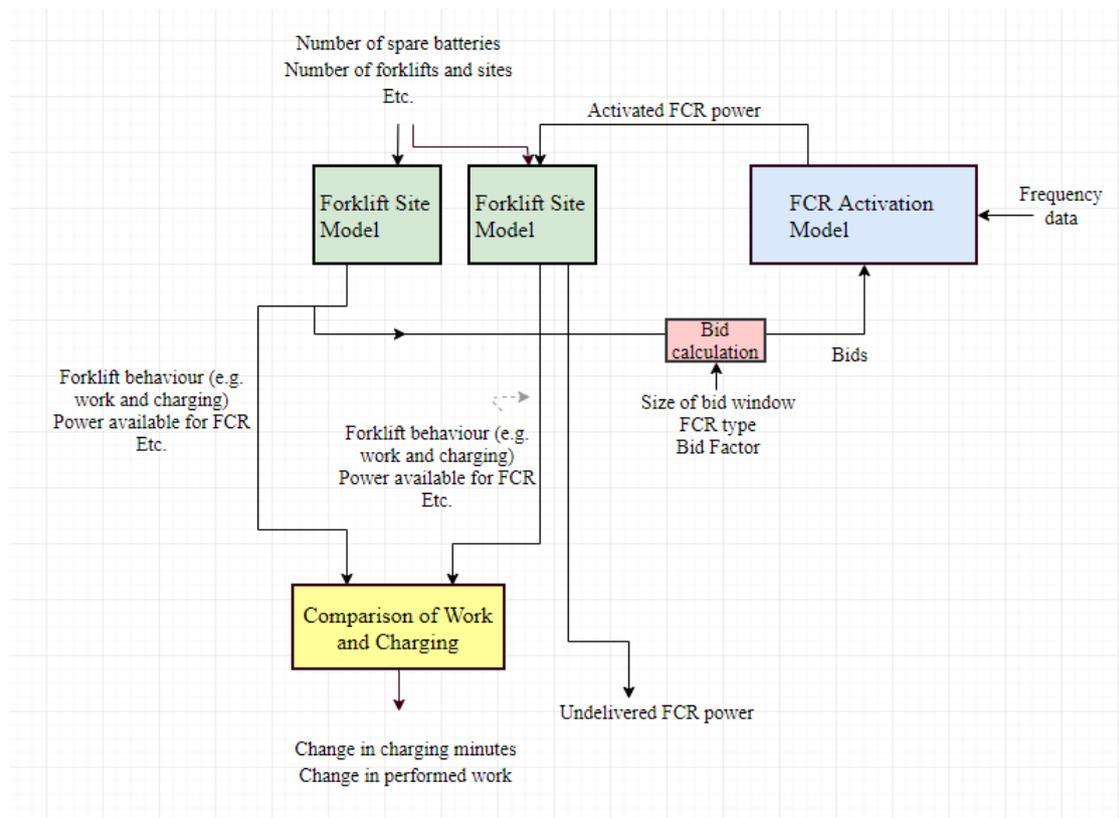
**Figure 3.1:** Flow chart illustrating the simulation model structure.
