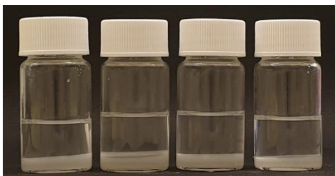
Figure 14. Reference, CC^{4.5}A^{0.5} -CA-9.8 + ethyl acetate + dispersant F, CC^{4.5}A^{0.5} -CA-9.8 + ethyl acetate + dispersant D and CC^{4.5}A^{0.5} -CA-9.8 + ethyl acetate + dispersant I.
