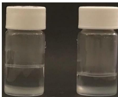
Figure 29. From left to right: CC^5 -CAC-2.5 in toluene, CC^5 -CAC-2.5dried with PEG present in toluene
