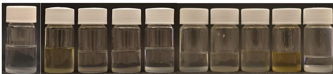
Figure 24. REF CC 5 -CAC-2.5 powder in toluene using dispersant A, B, C, D, E, F, G, H, I.
