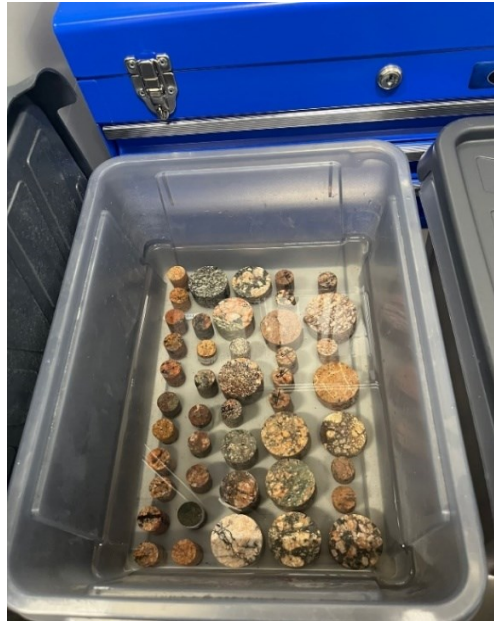
Figure 5: Selected saturated crystalline rock specimens used for ultrasonic testing. Source: Oy Rock Physics Ltd.
