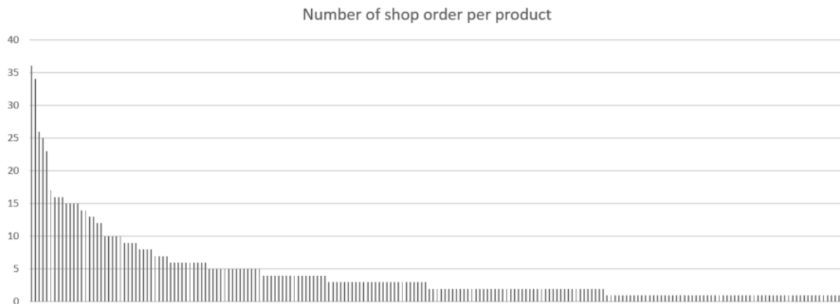
Figure 4.1: Pareto diagram of the number of shop orders between 2016-01-01 - 2019-12-31. Each bar represents one unique type of product.
