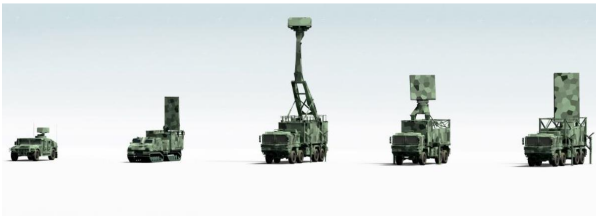
Figure 4.3. Examples of systems assembled in the Installation hall. Note that the vehicles are not produced by TCC and is provided by the customer to either directly assemble the radar system on it or provide portable solutions with the roll on-roll off containers or swap bodies.
