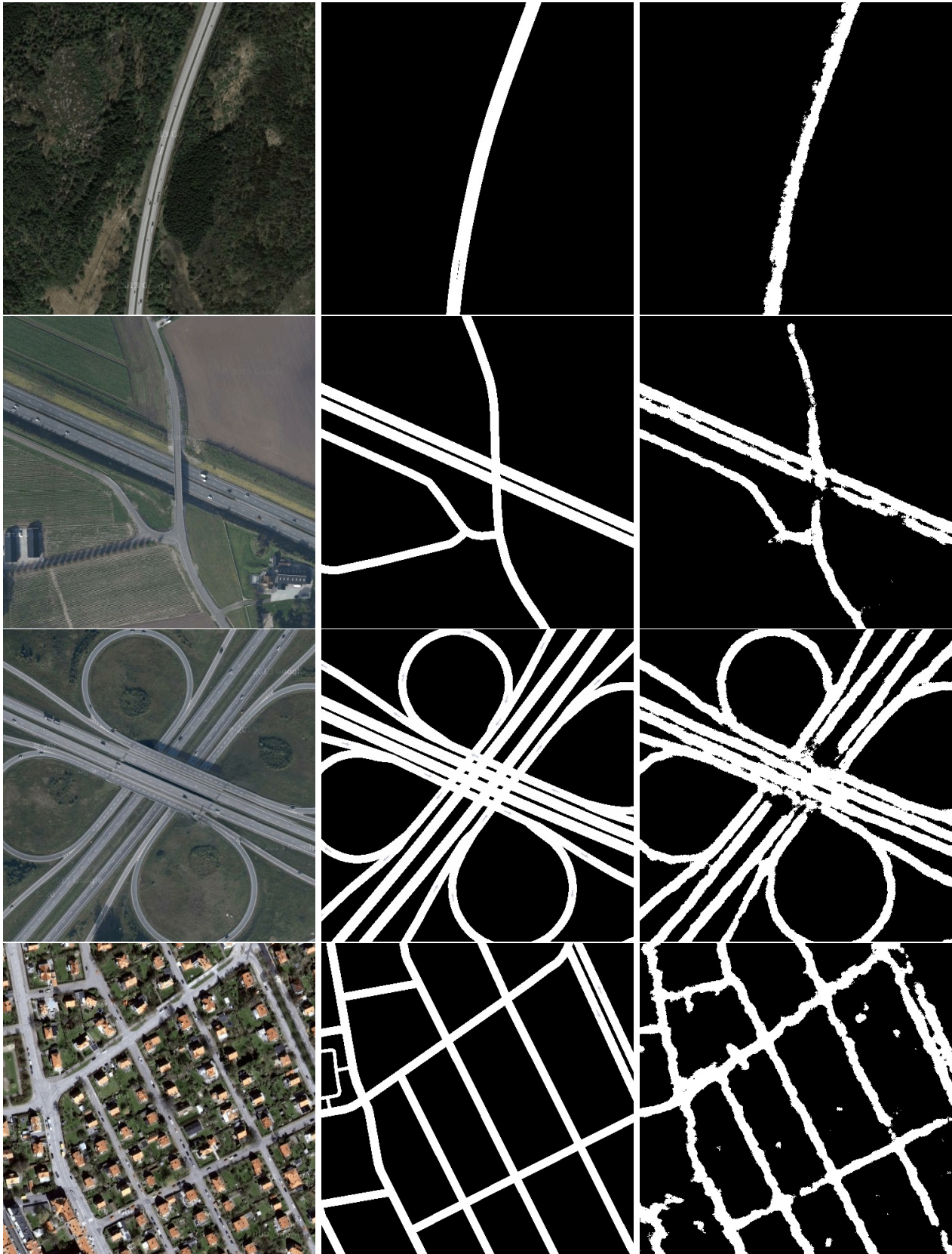
Figure 5.1: The four aerial images used for evaluating the road extraction system. In the left column are the unprocessed Google Map images, in the middle column are the gold images taken from Google Maps and in the right column are the predicted road maps. The images will be referred to as, from top to bottom, "Lindome", "Lomma", "Malmö" and "Helsingborg".
