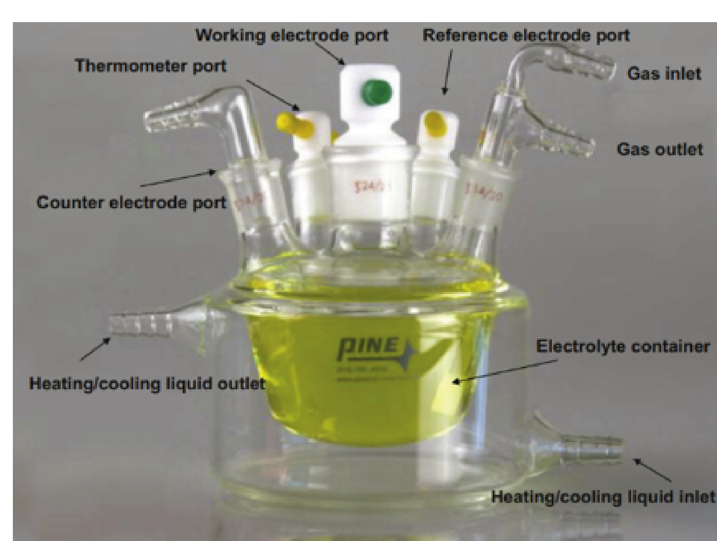
Figure 2: Schematic of the three-electrode cell for RDE measurements [3].
