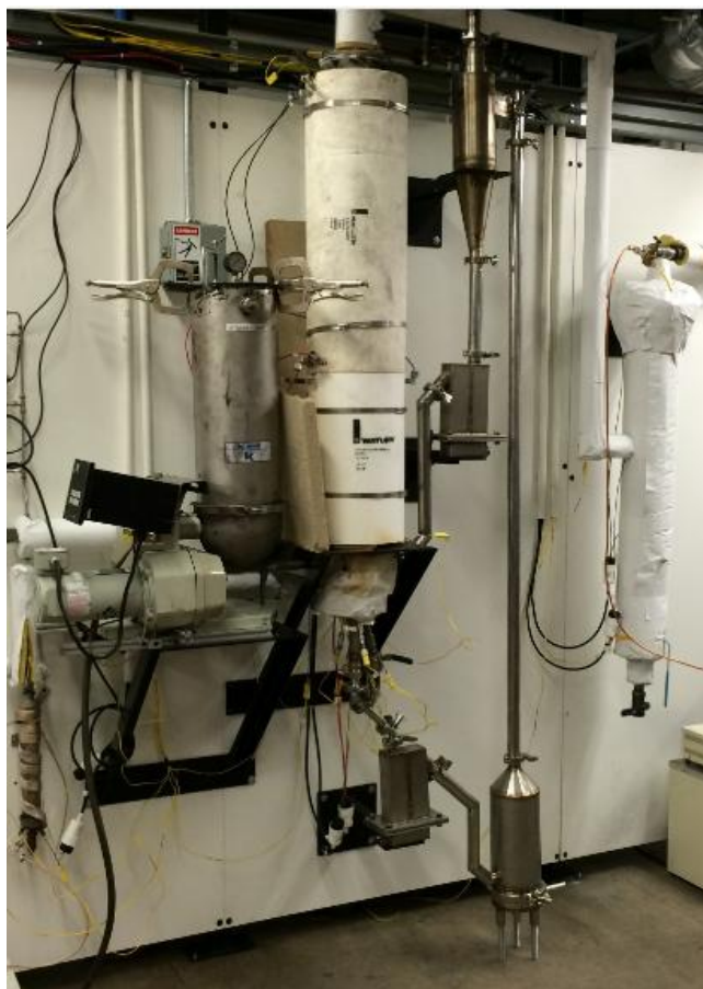
Figure 12. The system in reality. To the left a solid fuel feeder has been installed and to the right there is a char filter. On the outside of the fuel reactor heaters have been added.
