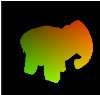
Image 33: This image shows an elephant model rendered using the manual vPos shader. As can be seen, the color (red and green channels) correctly represents the uv-coordinates for a fullscreen quad. Since 0,0,0 = black, 1,0,0 = red, 0,1,0 = green, 1, 1,0 = yellow.
