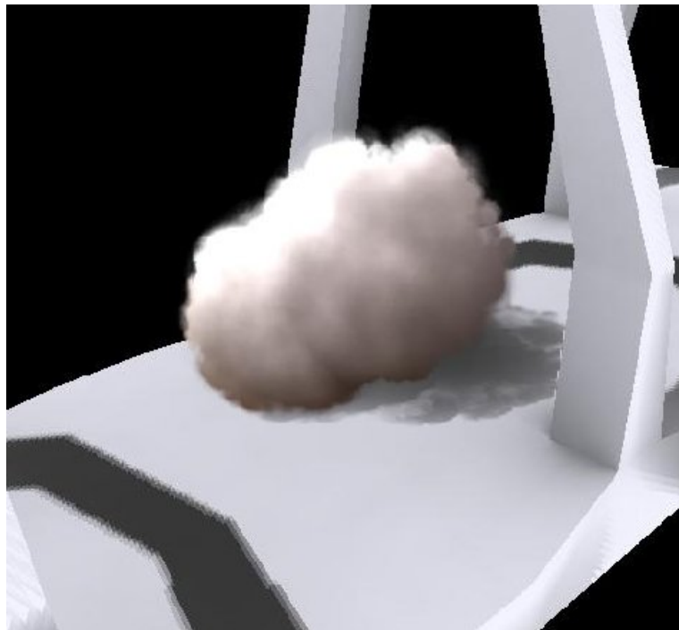
Image 38: Here shadows are tested. Both the scene and the smoke casts shadows. The smoke shadows are simply projected while the scene is using real exponential shadow mapping.
