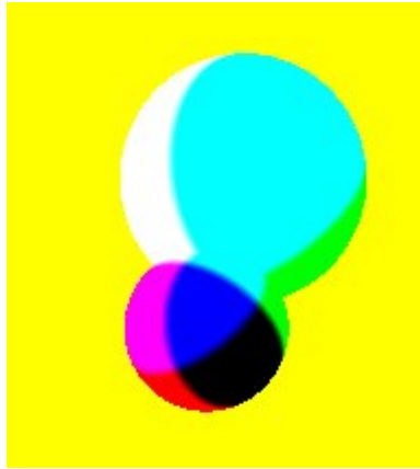
Image 15: This image shows the world position of the pixels of two particles. This world position have been reconstructed from the depth of two raytraced spheres in a previous pass. The position coordinates have simply been written to the screen and naturally colors the spheres. 0,0,0 \rightarrow white, 1,1,1 \rightarrow black, 1,0,0 \rightarrow red, and so on.
