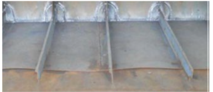
(b) Stiffened panel on the inside of ship hull.
