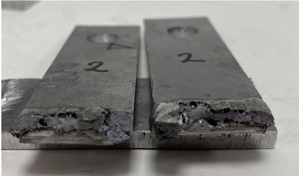
Figure 20, *Tensile testing of ENAB 44300 (V-HPDC) welded to ENAB 44300 (V-HPDC)*
