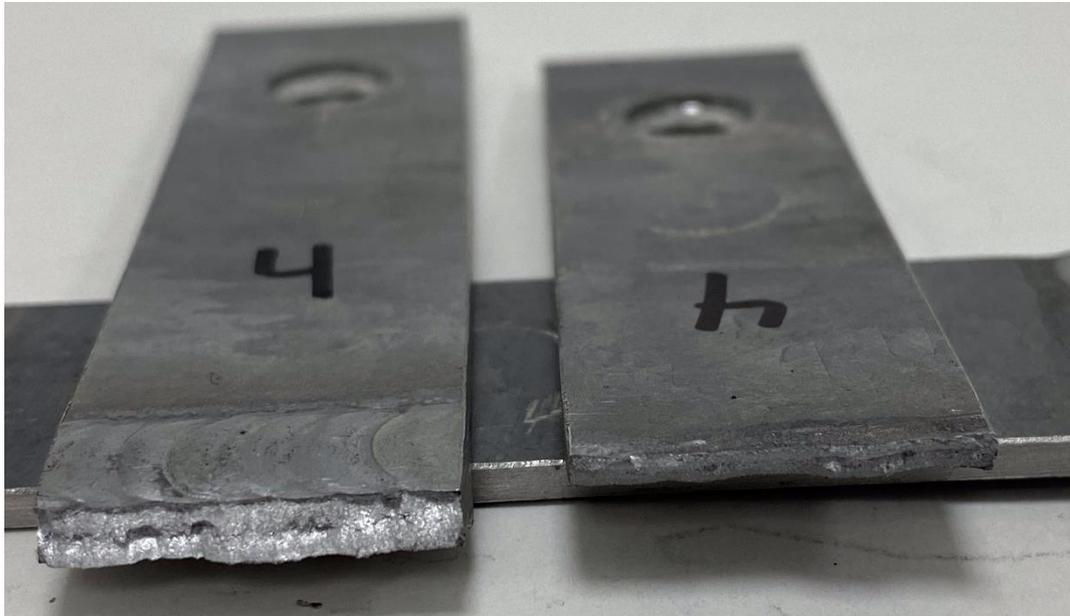
Figure 22, *Tensile testing of ENAB 42000 (rheocasting) welded to ENAB 42000 (rheocasting)*
