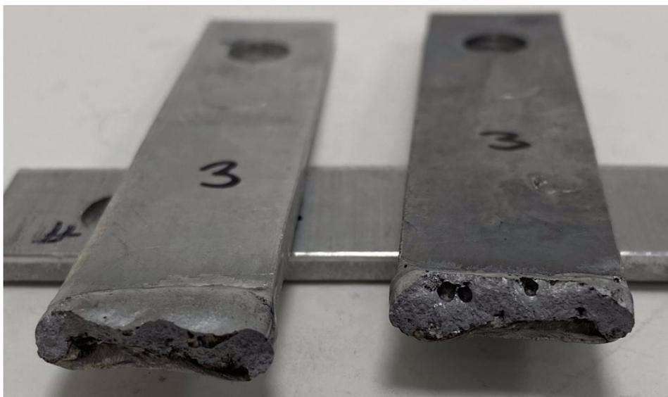
Figure 18, Tensile tested *EN-AW 6063-T6 (4 mm) welded to ENAB 44300 (V-HPDC)*
