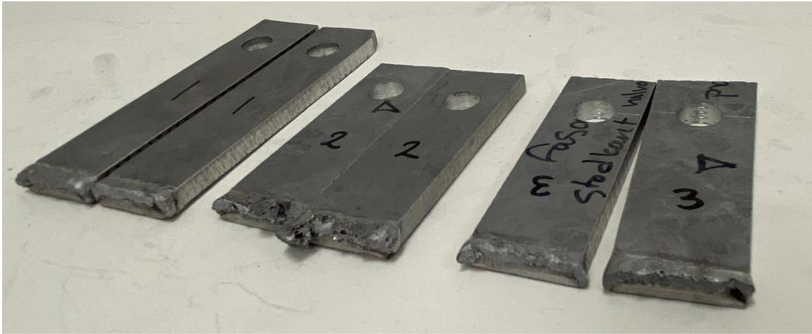
Appendix 24, *Tensile testing of ENAB 44300 (V-HPDC) welded to ENAB 44300 (V-HPDC)* 2
