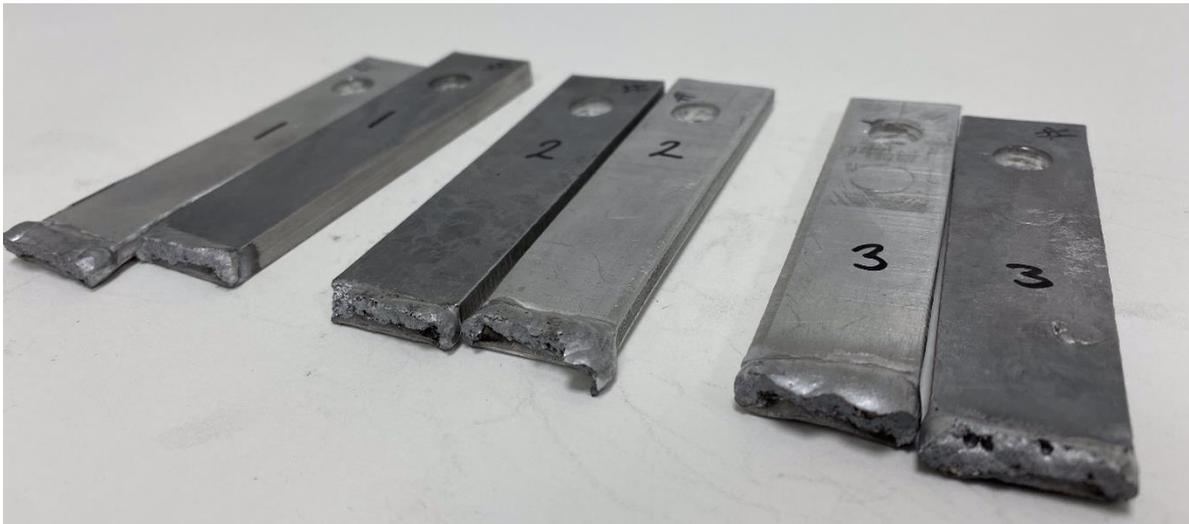
Appendix 21, *Tensile tested EN-AW 6063-T6 (4 mm) welded to ENAB 44300 (V-HPDC) 2*
