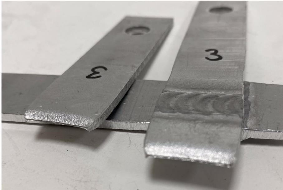
Figure 14, *Tensile testing of welded EN-AW 6063-T6 (3mm) to EN-AW 6063-T6 (3mm)*
