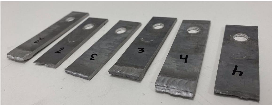
Appendix 27, *Tensile testing of ENAB 42000 (rheocasting) welded to ENAB 42000 (rheocasting) 2*
