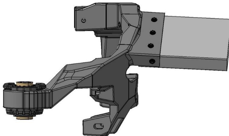
Figure 12, *Example of an FDS- and a combined FDS-adhesive joint*
