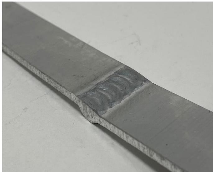
Figure 13, *Two pieces of EN-AW 6063-T6 (3mm) welded together*
