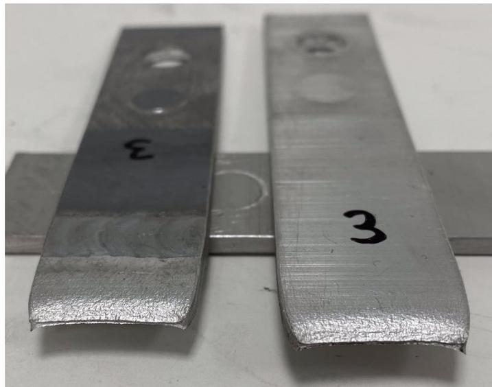
Figure 16, Tensile testing of *EN-AW 6063-T6 (3 mm) welded to ENAB 42000 (rheocasting)*
