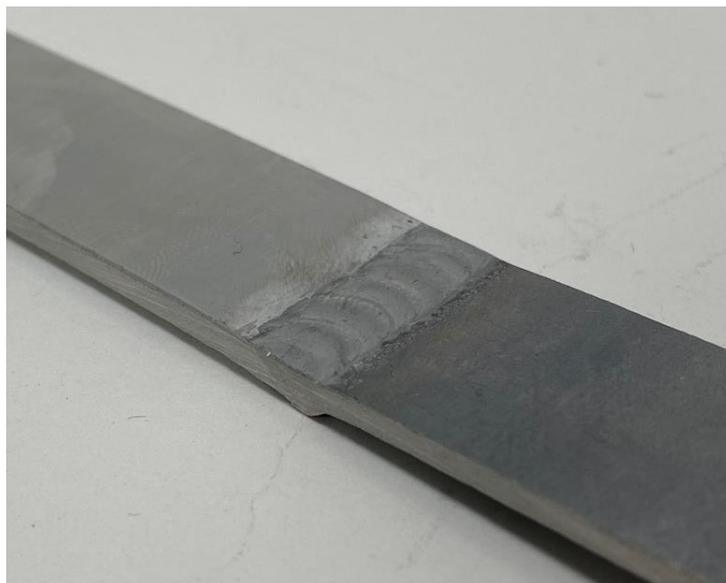
Figure 15, *EN-AW 6063-T6 (3 mm) welded to ENAB 42000 (rheocasting)*
