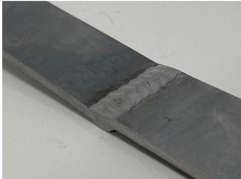
Figure 21, *Two pieces of ENAB 42000 (rheocasting) welded together*
