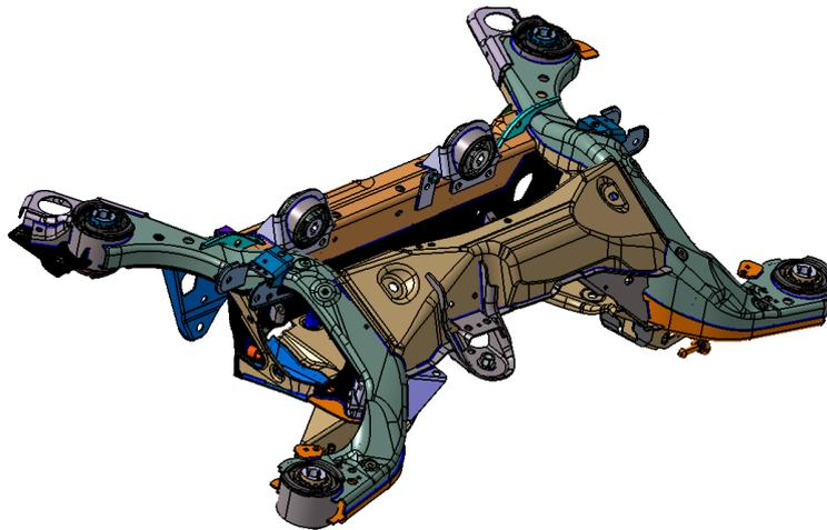
Figure 7, Existing stamped and welded steel subframe from an XC40
