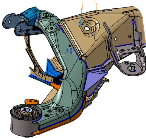
Figure 8, *Section of the existing subframe*
