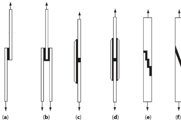
Figure 6, *Basic bonded joint designs: (a) single lap joint, (b) double lap joint, (c) single strap joint, (d) double strap joint, (e) stepped lap joint, and (f) scarf joint.* (Mallick, 2020)
