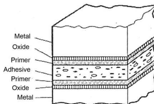
Figure 2, *Composite structure of typical metal-to-metal bonded joint* (Burt, 2018)
