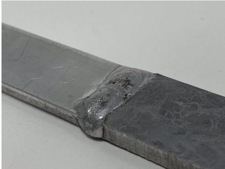
Figure 17, *EN-AW 6063-T6 (4 mm) welded to ENAB 44300 (V-HPDC)*
