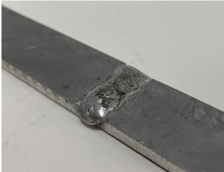
Figure 19, *Two pieces of ENAB 44300 (V-HPDC) welded together*
