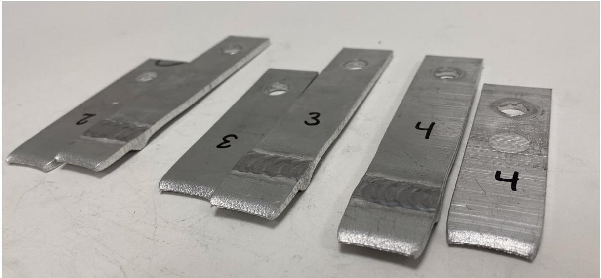
Appendix 15, *Tensile testing of welded EN-AW 6063-T6 (3mm) to EN-AW 6063-T6 (3mm) 2*
