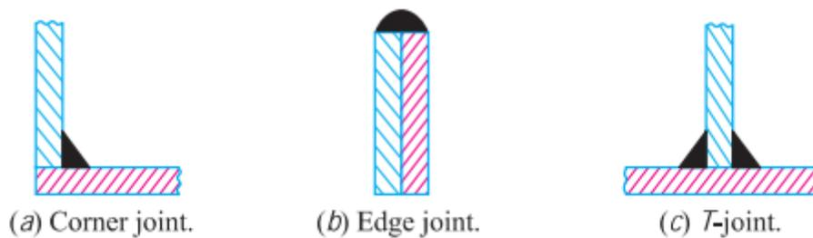
Figure 5, *Other types of welded joints.* (Khurmi & Gupta, 2005)
