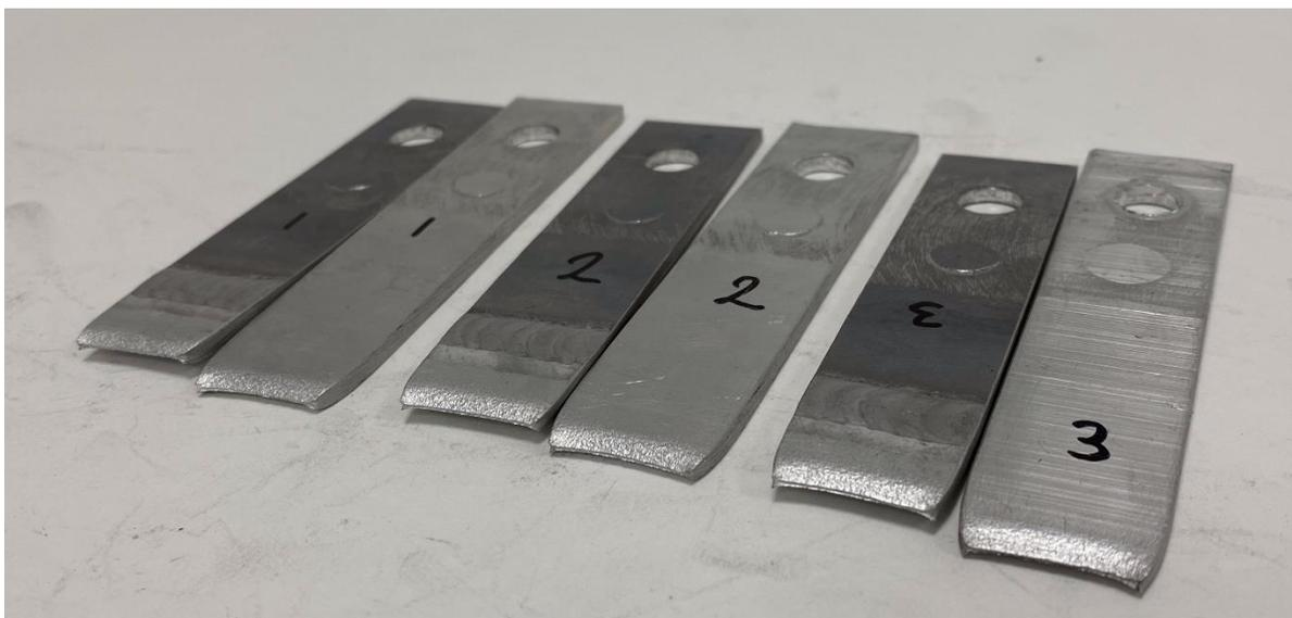
Appendix 18, Tensile testing of *EN-AW 6063-T6 (3 mm) welded to ENAB 42000 (rheocasting) 2*
