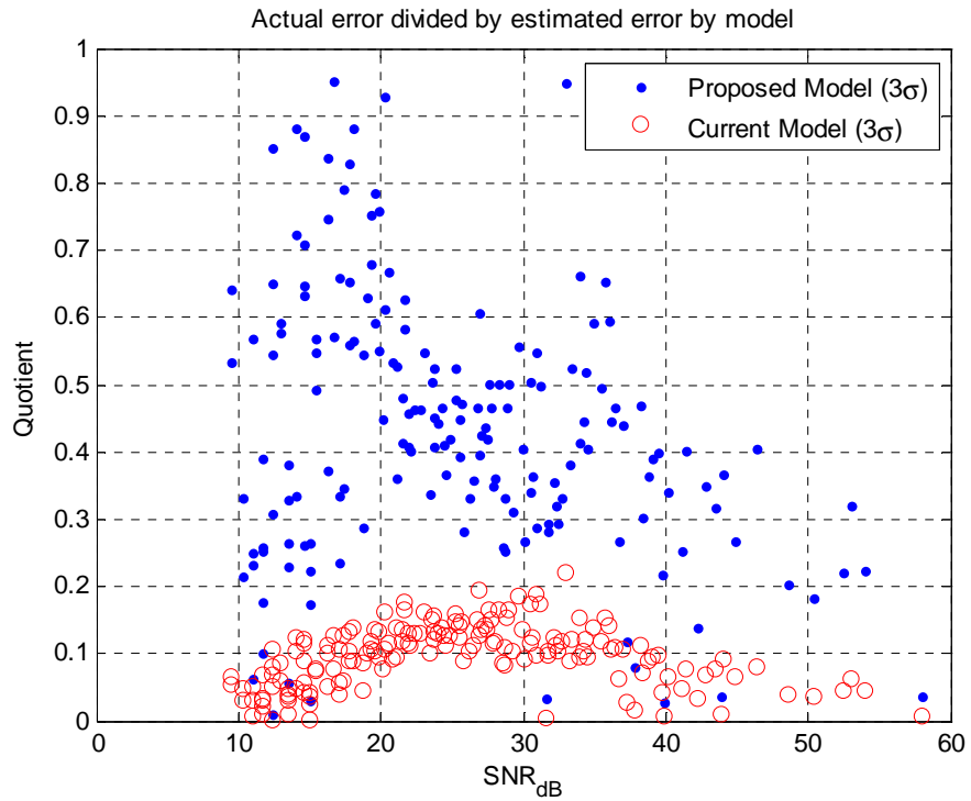
Figure 30 Quotient between the actual error and the estimated error from the 3\sigma model. A value above one indicates that the estimated accuracy is overoptimistic, a value below one is wanted. Plots are randomly chosen to illustrate the quotient.
